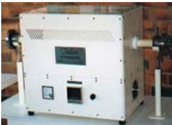
Figure 2.2 A photograph of a Tetlow Tube Furnace.
