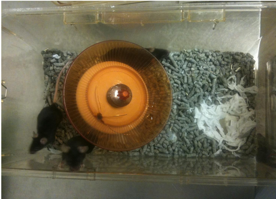
Figure 2-2 Housing for our mice. Mice placed in a cage along with a running wheel, which they have free access to. The bottom of the cage is lined with recycled paper, which is used as bedding material for the mice. The running wheels used were wirelessly connected to a USB-HUB and the amount of rotations that the wheel turns is recorded every 30 seconds.
