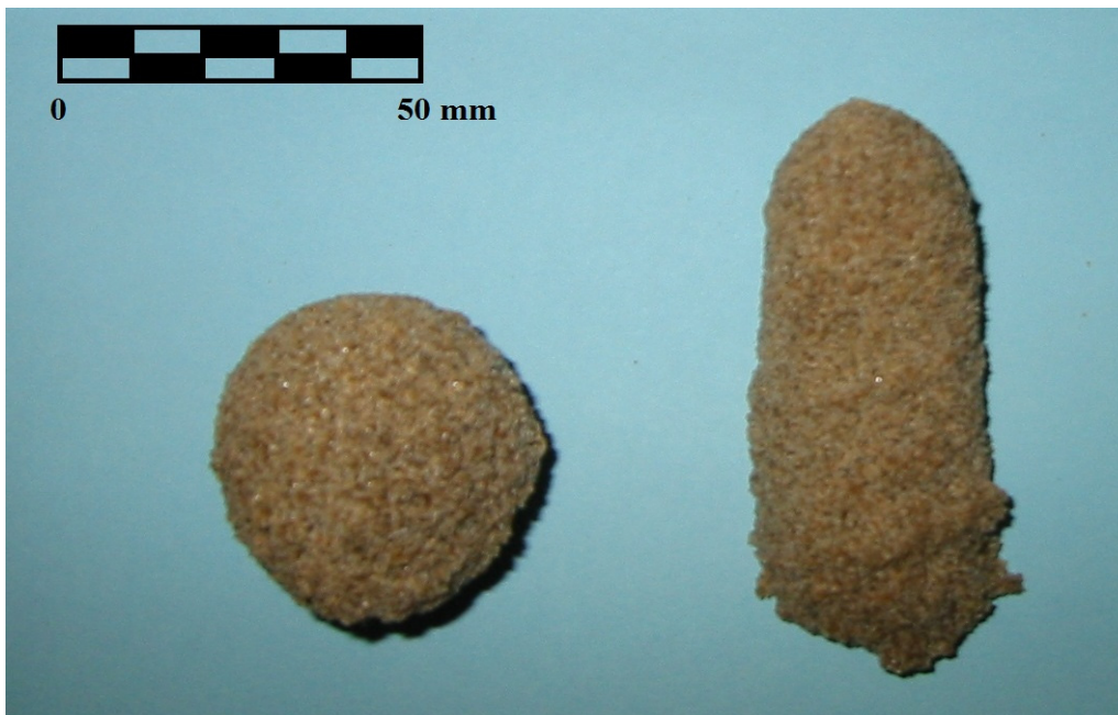
Figure 3.17. Extracted sand-resin lumps prior to trimming.
