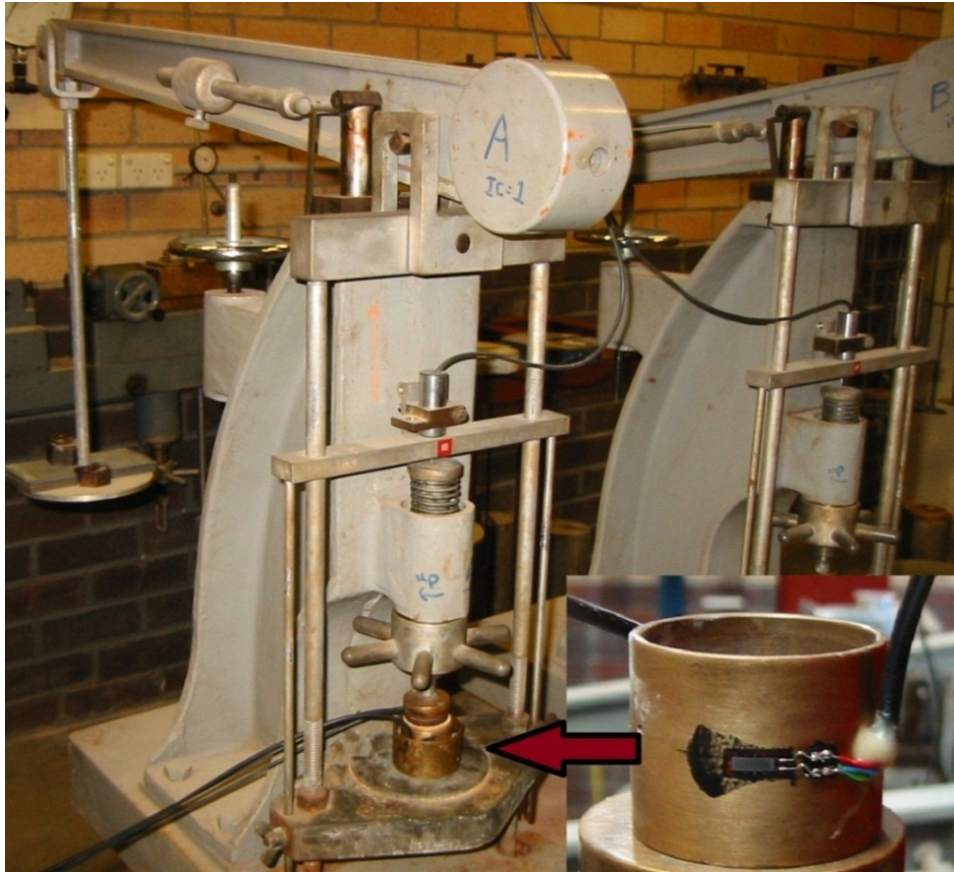
Figure 3.23. Set up of oedometer experiment for k_0 measurement
