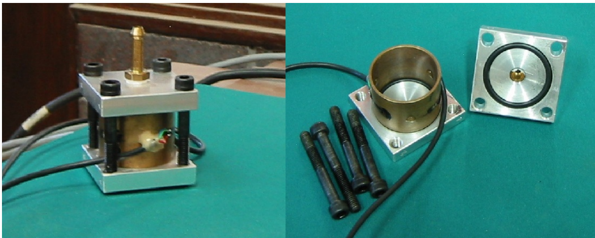
Figure 3.24. Set up of the oedometer cell with the caps used to seal the ring during calibration.
