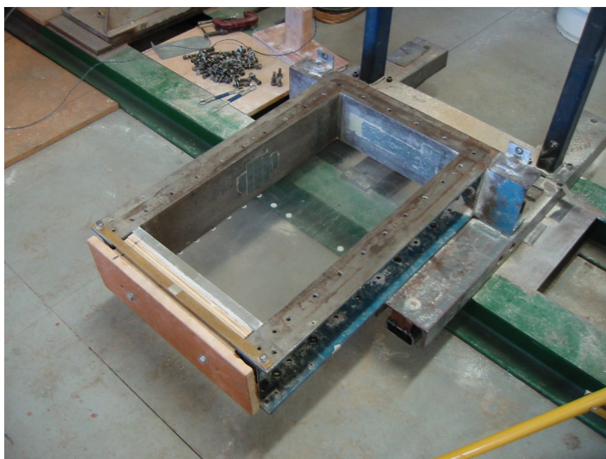
Figure 3.4. The soil container of small model Type 2 rotated through 90^\circ to the horizontal with its backside removed and top of the container plugged to facilitate sample preparation.
