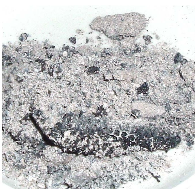
Figure 84: Corn cob ash calcined at 600°C in open container
