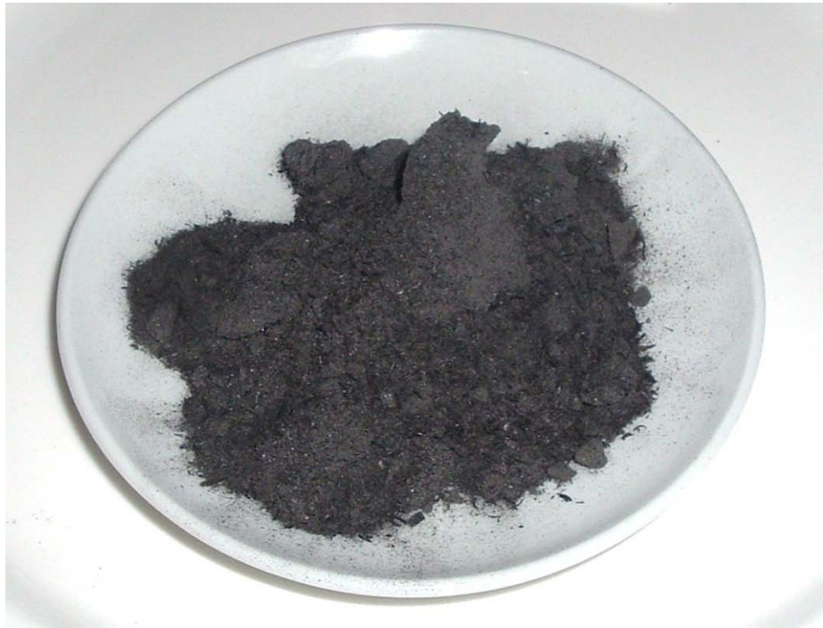
Figure 65: Bagasse ash (number 12 boiler belt) calcined at 600°C
