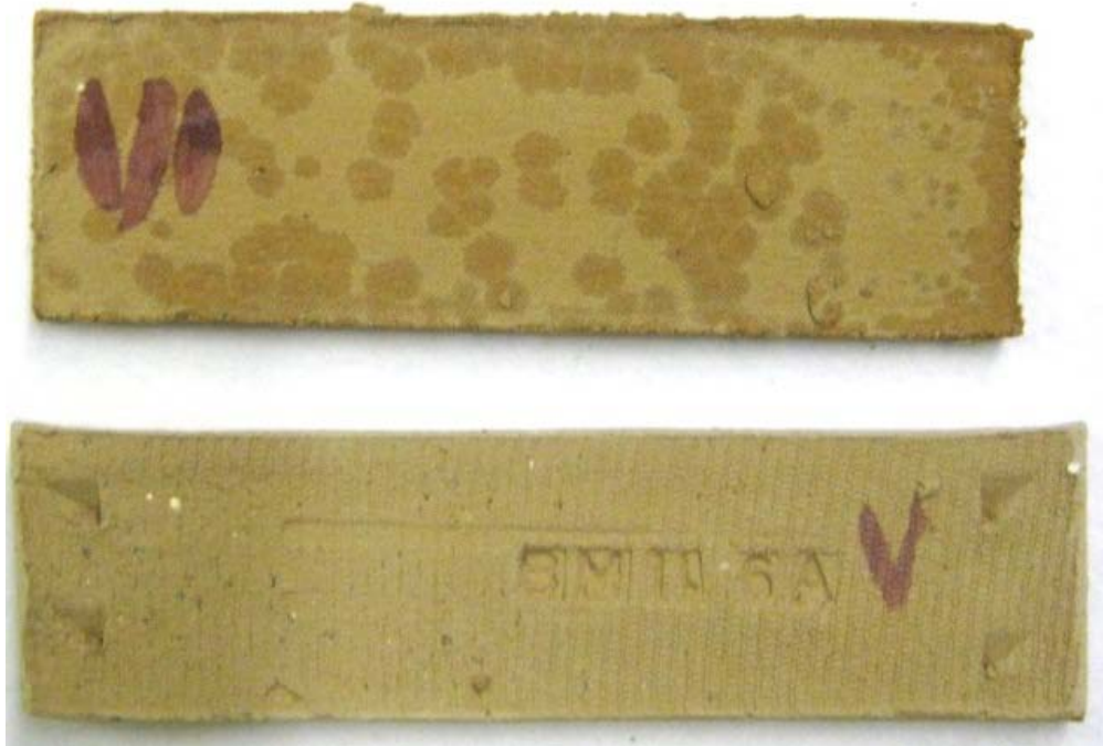
Figure 429: Efflorescence comparison of BM11.6 (top) and BM11.6A treated with barium carbonate to reduce efflorescence
