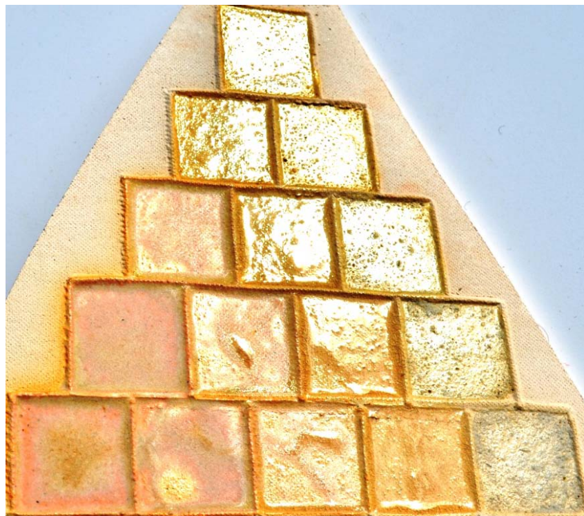
Figure 452: Low-fire 2 triaxial after firing to 1000°C showing reflectivity
