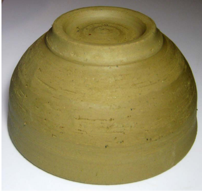
Figure 151: Turned foot ring on bowl thrown from 100% Marulan tailings
