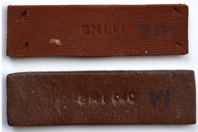
Figure 332: BM1.14 (top) and BM1.14C fired to 1100°C
