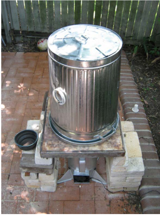
Figure 282: Rubbish bin kiln in position
