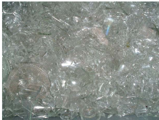
Figure 111: Clear glass bottles crushed in the Bottlecyclor crusher
