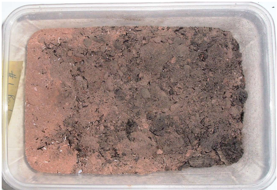
Figure 66: Bagasse ash (number 12 boiler belt) calcined at 700°C
