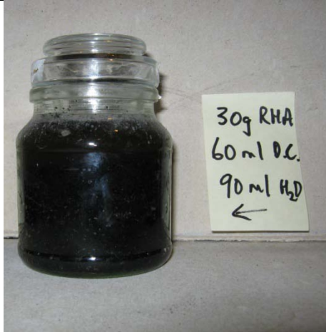
Figure 295: Mix 2: 30g RHA, 60ml Drain Clear, 90ml Water
