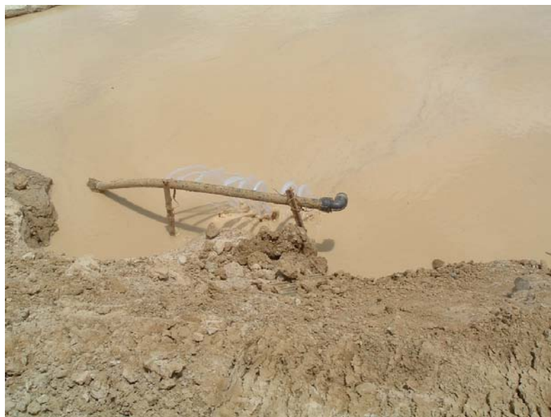
Figure 125: Flocculated Bungendore tailings settling pond
