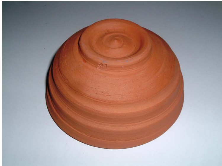
Figure 158: Bowl of 50% Bungendore, 50% Marulan tailings fired to 800°C
