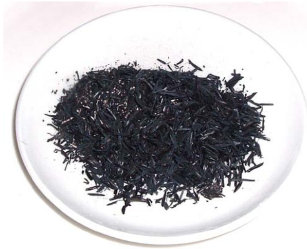
Figure 73: RHA calcined at 600°C
