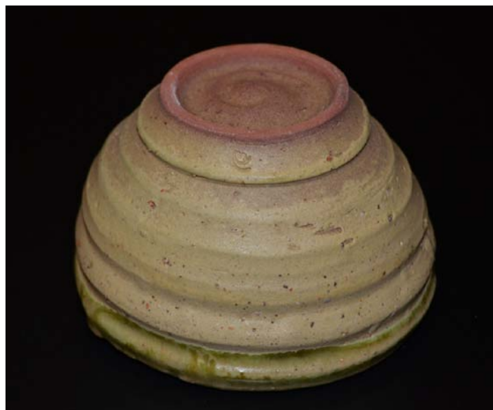
Figure 496: Bowl 3: BM11.6A, 940°C. Self-glazed exterior, unglazed foot ring. Glaze 17.4 (rim)
