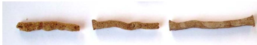
Figure 274: Samples BM2.4–BM2.6 after firing to 800°C
