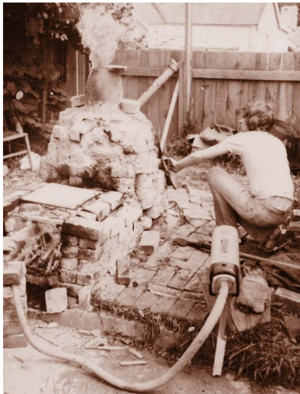
Figure 19: Salting a suburban coal-fired kiln, Dunedin, New Zealand, 1980
