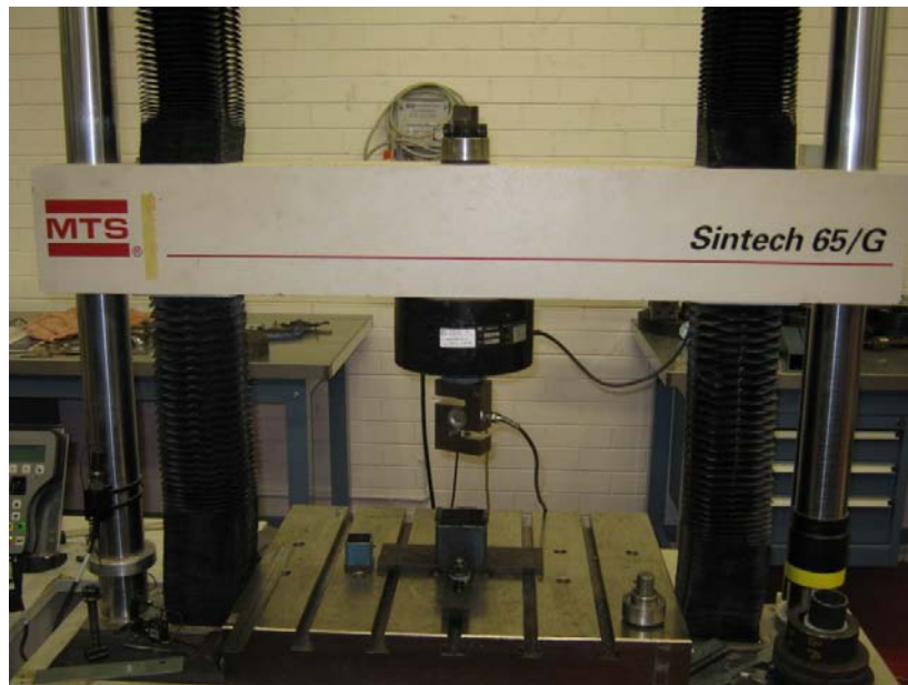
Figure 434: Apparatus for stress tests
