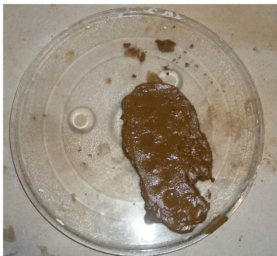
Figure 214: BM2.2 one day after microwaving to remove moisture
