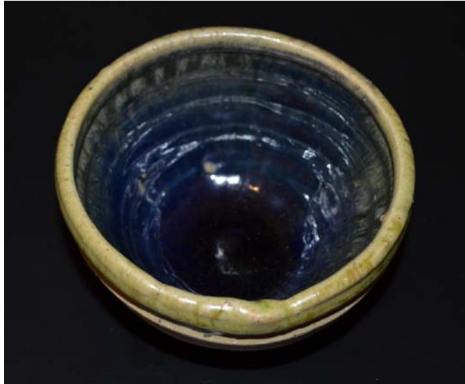
Figure 495: Bowl 3: BM11.6A fired to 940°C. Glazes 17.2 (interior) and 17.4 (rim)
