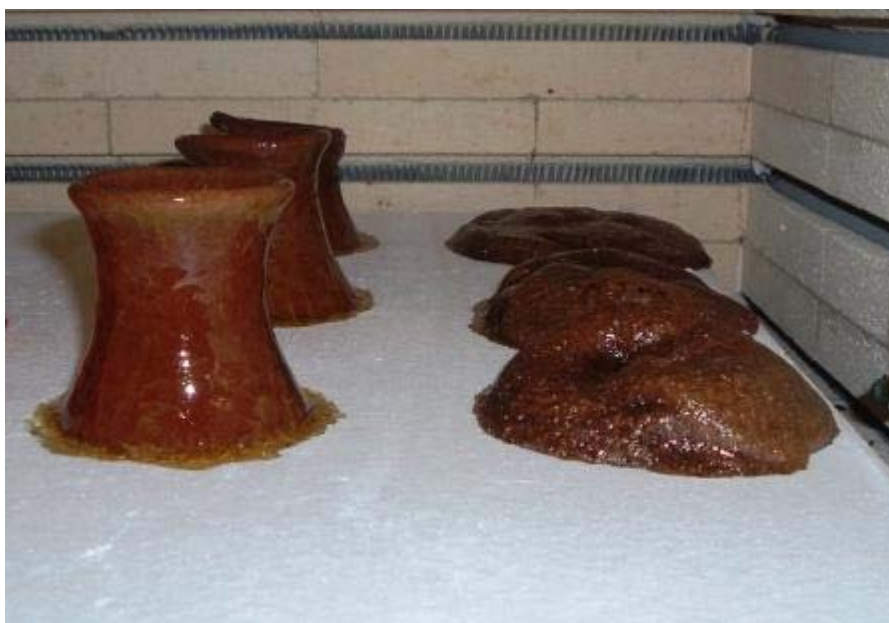
Figure 328: Melted towers at 950°C: BM2.7 (left) and BM2.9
