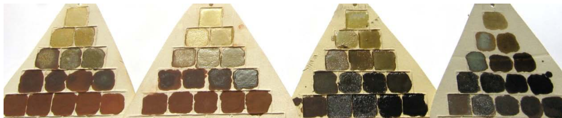
Figure 437: Triaxial BM11: Glaze/engobe tests at (l to r) 1000, 1100, 1200 and 1280°C
