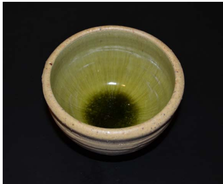
Figure 490: Bowl 1 thrown from BM11.6A, fired to 940°C, Glaze 17.4
