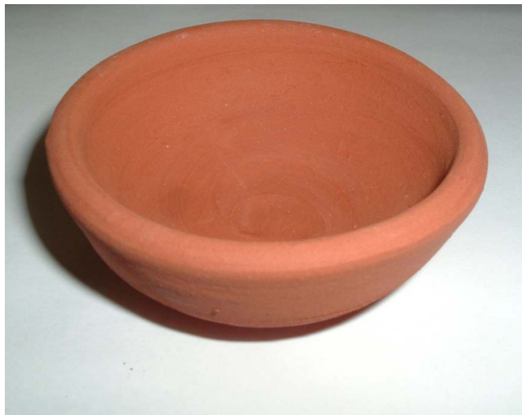
Figure 156: Bowl thrown from Bungendore tailings fired to 800°C
