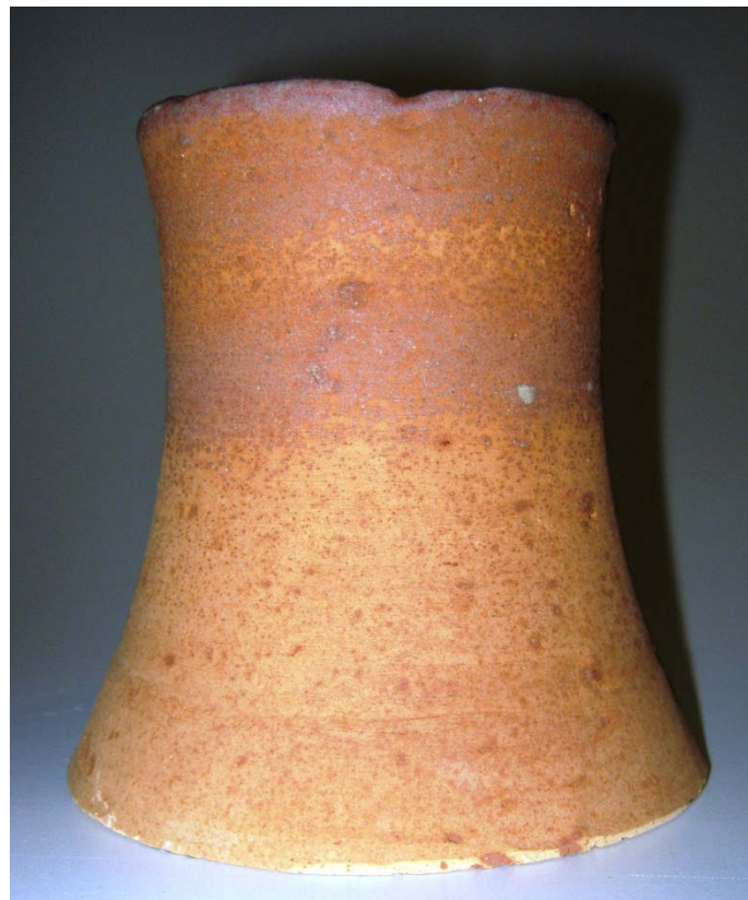
Figure 508. BM11.6B 50: 50 WMF blend fired to 900°C. 15x20cm
