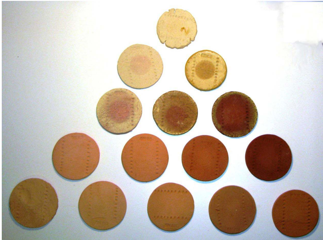
Figure 346: All BM11 sample discs fired to 900°C: Extent of efflorescence and self-glazing
