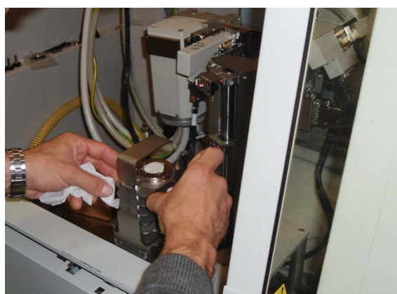
Figure 301: Loading samples into rack
