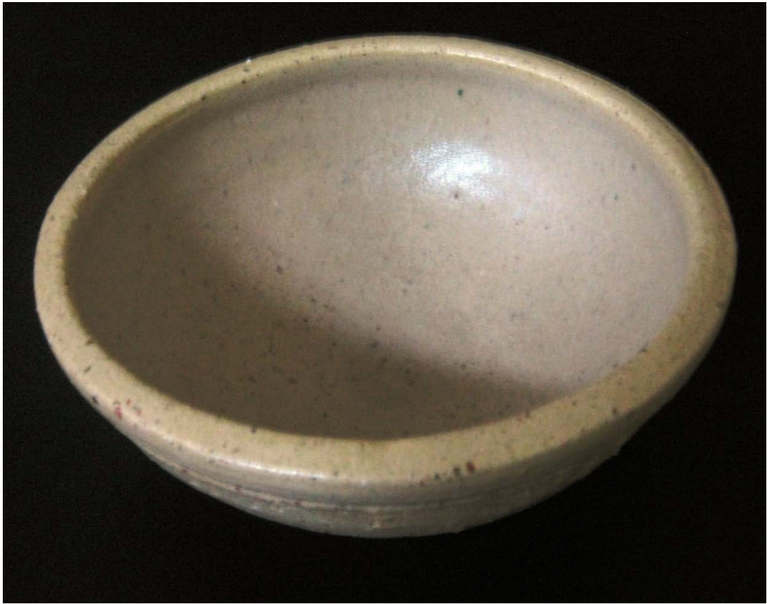
Figure 506: Bowl 6: BM11.6B, 950°C. Glaze 19 without colourant addition
