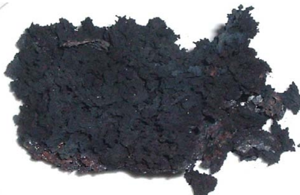
Figure 95: Corn seeper sludge calcined at 600°C
