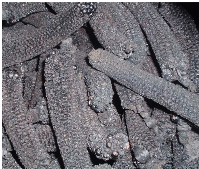
Figure 85: Corn cob ash charcoal from calcining at 600°C in closed container
