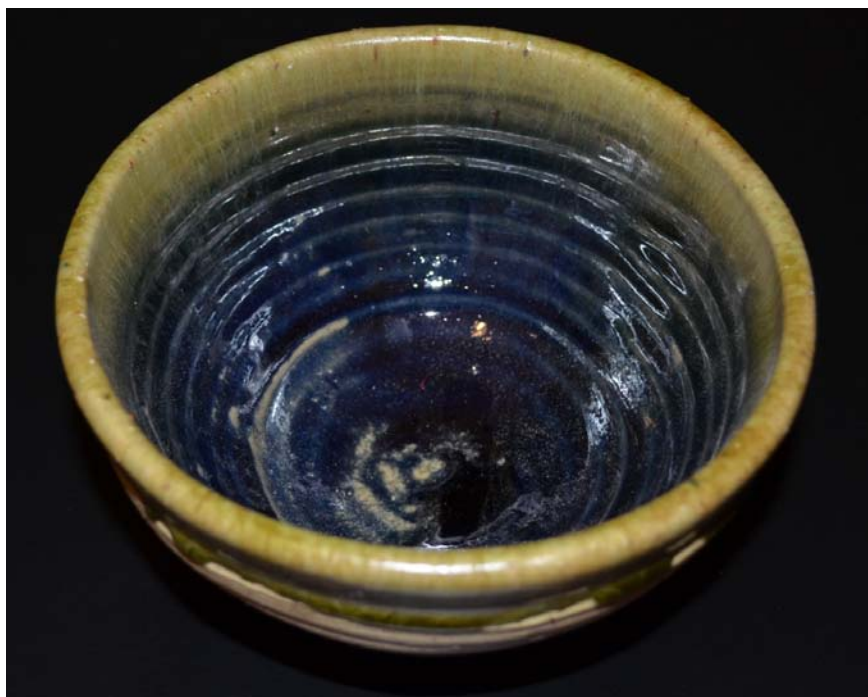
Figure 498: Bowl 4: BM11.6A fired to 950°C. Glazes 17.2 (interior) and 17.4 (rim)
