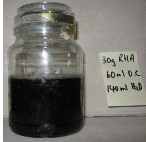
Figure 296: Mix 3: 30g RHA, 60ml Drain Clear, 140ml Water
