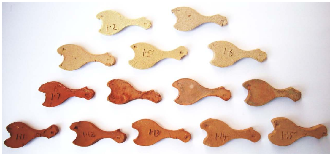
Figure 256: Triaxial BM1. Fired to 800°C. Samples 2-15
