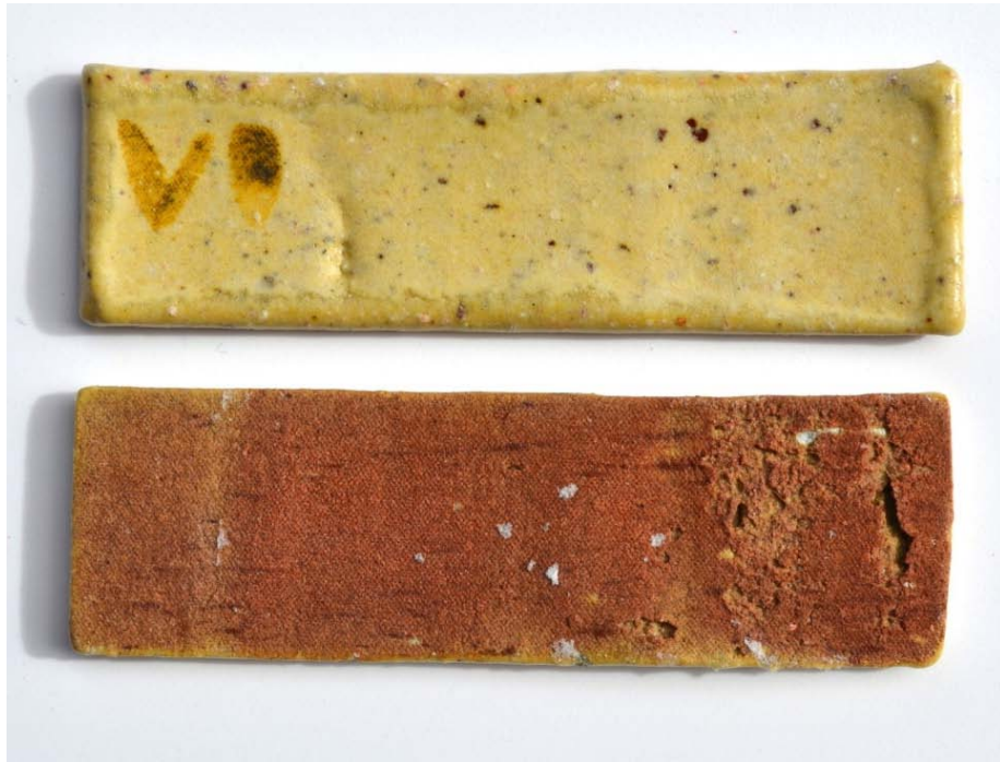
Figure 431: BM11.6 self-glazed exposed side (top) and unglazed protected side after firing to 1050°C
