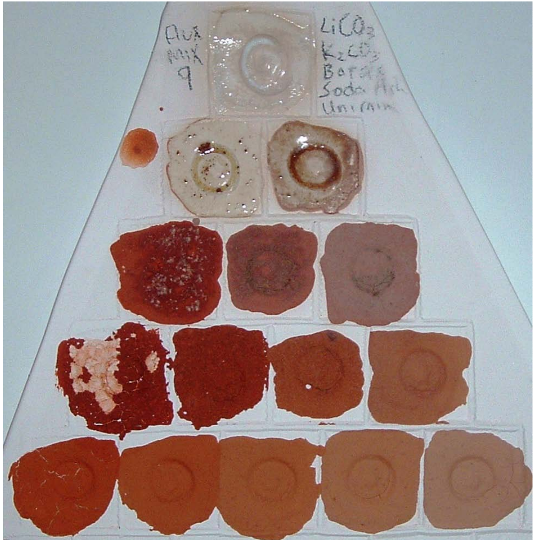
Figure 321: BM2 Triaxial fired to 900°C
