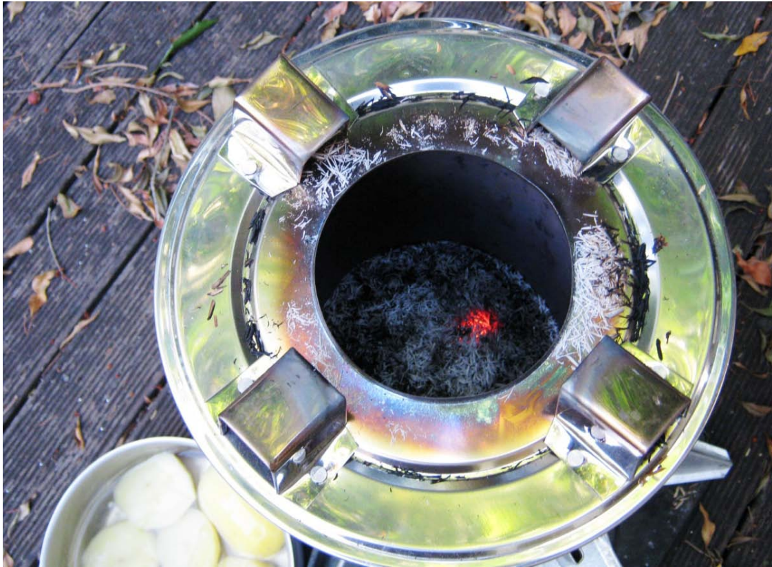
Figure 277: Burnt rice husk in biomass gasifier
