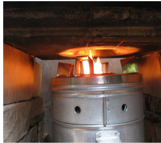
Figure 289: Cobs burning without primary air
