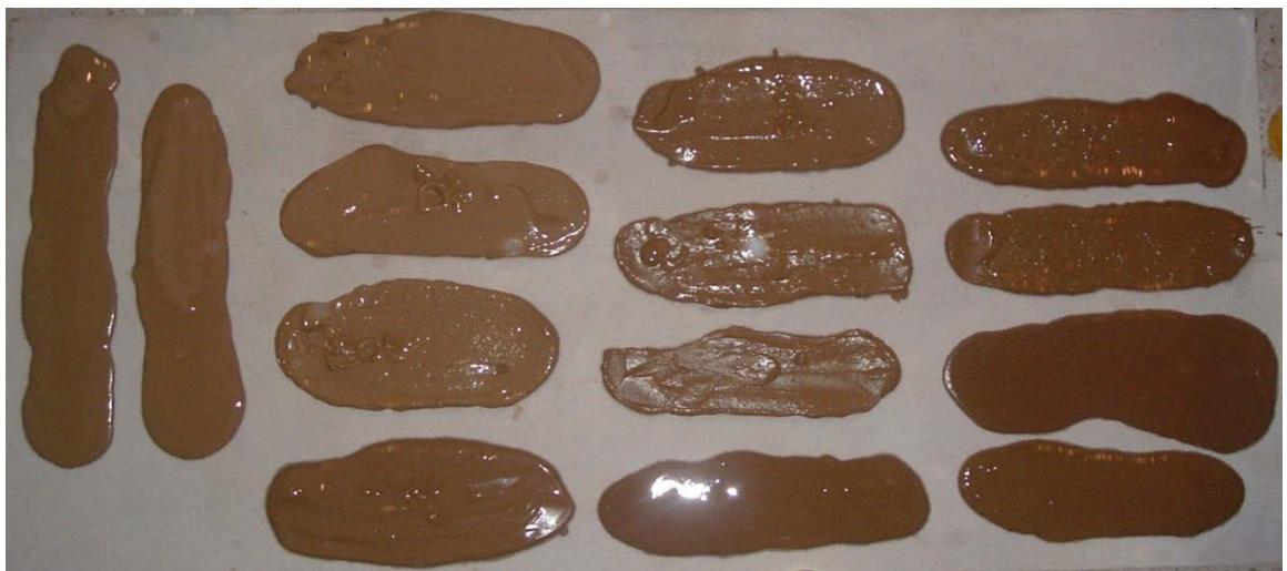
Figure 163: Triaxial sample slips drying before kneading and bagging
