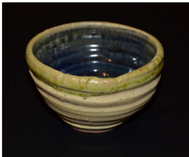
Figure 494: Bowl 3: BM11.6A fired to 940°C. Glazes 17.2 (interior) and 17.4 (rim)
