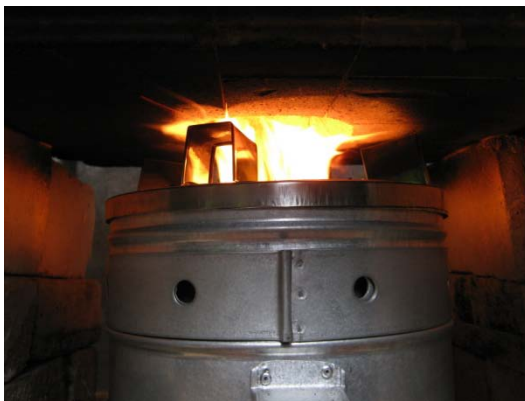
Figure 290: Cobs burning with primary air
