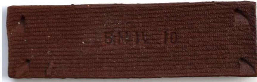
Figure 427: BM11.10 fired to 1100°C: Protected surface
