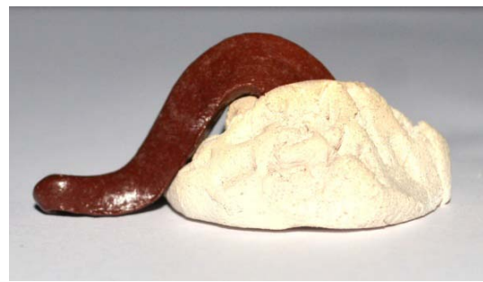
Figure 488: Cone 08 after reading 950°C
