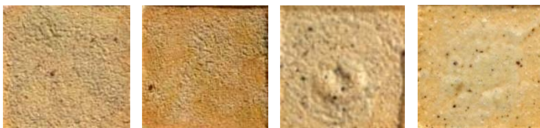
Figure 453: Low-fire corn/sugarcane ash at (l to r) 950, 1000, 1050 and 1100°C
