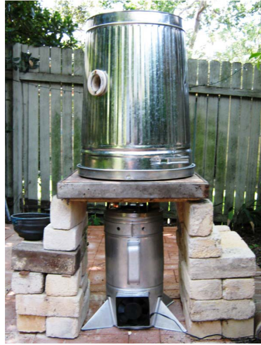
Figure 283: Rice husk stove in position
