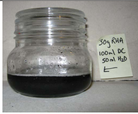
Figure 294: Mix 1: 30g RHA, 100ml Drain Clear, 50ml Water.
