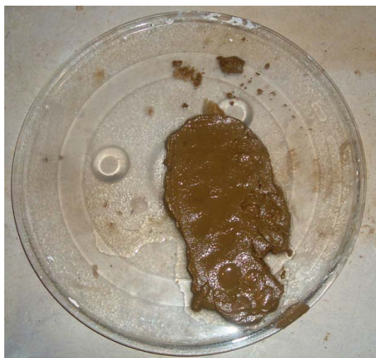
Figure 215: BM2.2 three days after microwaving, showing liquid run-off
