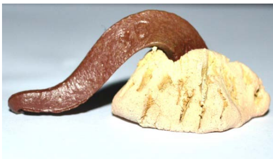
Figure 487: Cone 08 after reading 940°C
