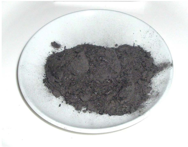
Figure 56: Bagasse ash (number 1 boiler belt) calcined at 600°C
