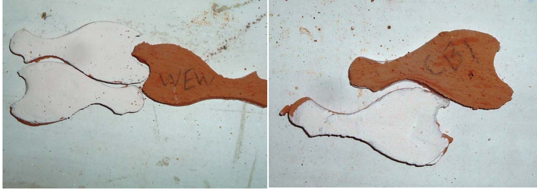
Figure 318: WEW engobe applied to BM1.13 bisque and fired to 950°C (unglazed)
