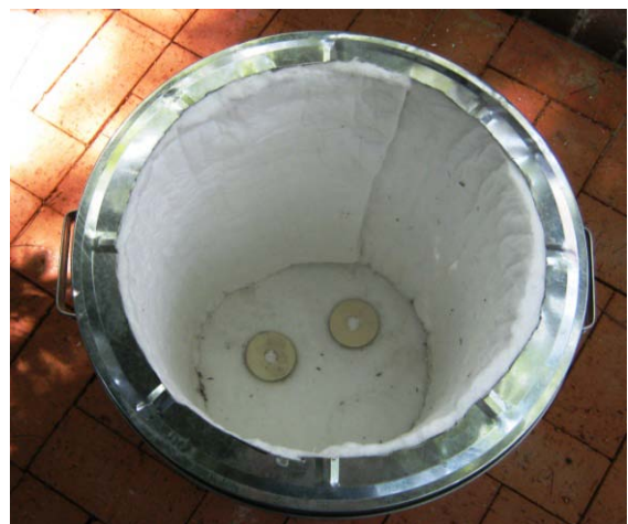
Figure 281: Secured fibre blanket
