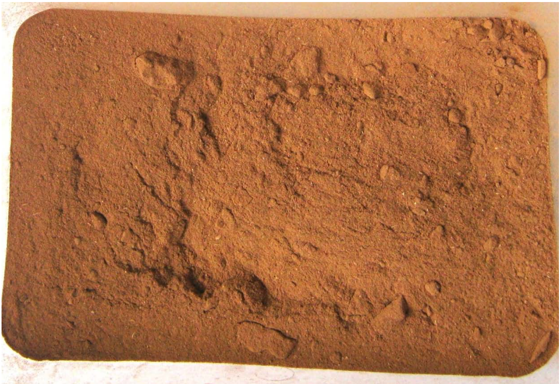
Figure 68: Bagasse ash (number 12 boiler belt) calcined at 900°C
