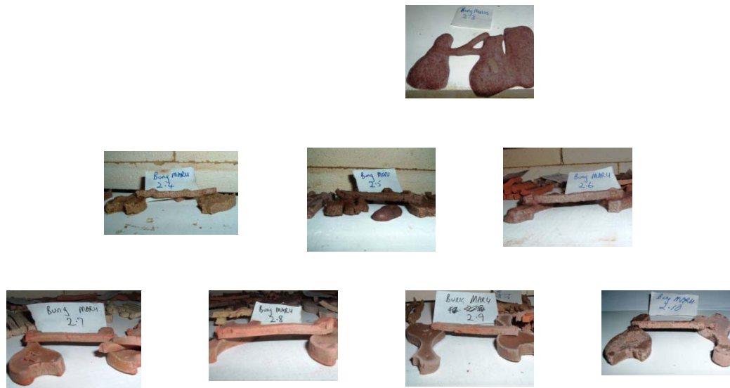
Figure 264: Triaxial BM2. Slump tests fired to 800°C: samples BM2.3–BM2.10
