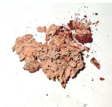
Figure 96: Corn seeper sludge calcined at 700°C
