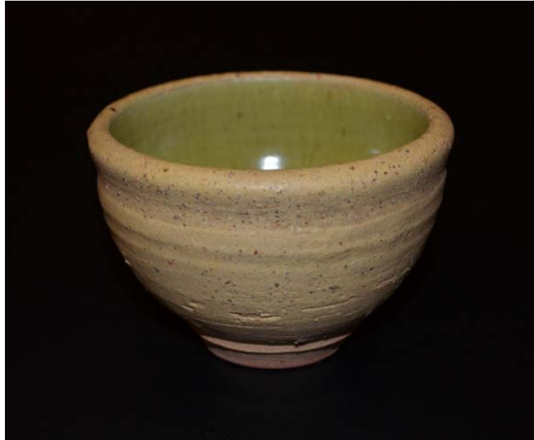
Figure 489: Bowl 1 thrown from BM11.6A, fired to 940°C, Glaze 17.4
