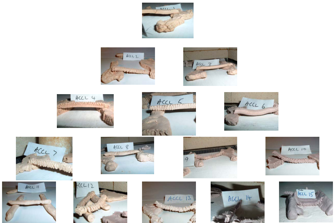
Figure 246: ACCL Triaxial slump tests after firing to 800°C
