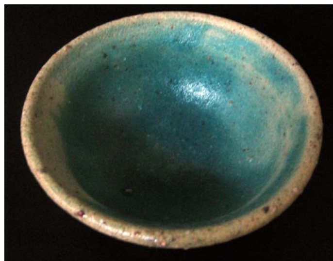
Figure 507: Bowl 7: BM11.6B, 950°C. Glaze 19 with 4% copper carbonate
