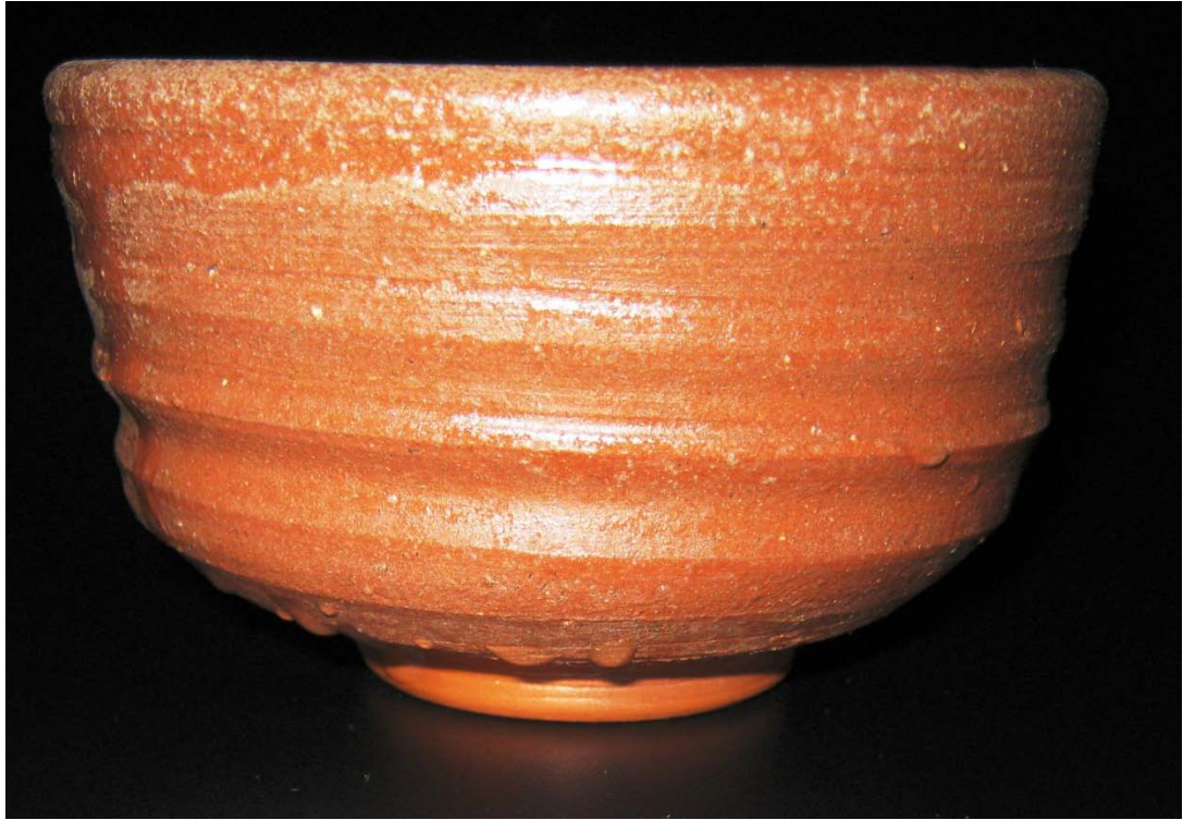
Figure 326: BM2.2 glaze on 800°C bisque BM1.13 bowl, seeping after being fired to 900°C, filled with water, and left to stand overnight
