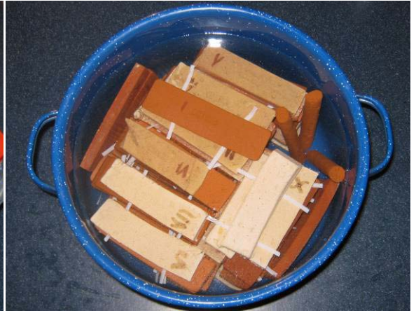
Figure 372: Dried and fired test bars soaking in distilled water
