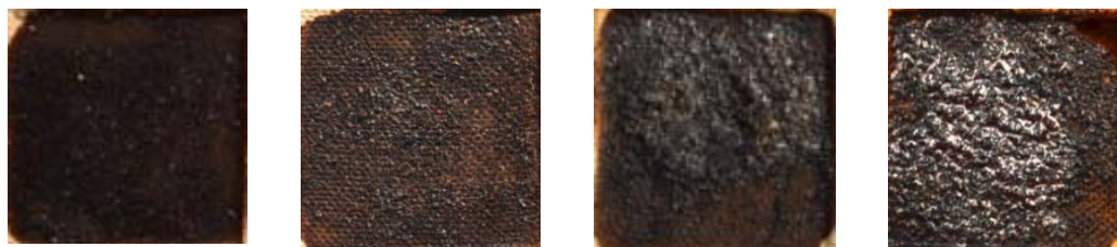
Figure 443: Low-fire corn ash 1 at (l to r) 950, 1000, 1050 and 1100°C
