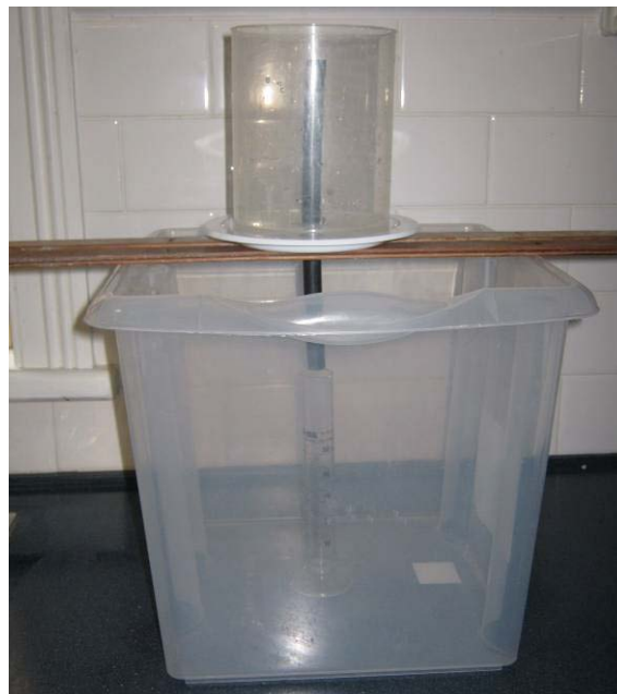
Figure 373: Apparatus for determining volume of fired bars using Archimedes' principle
