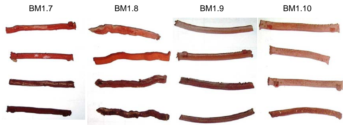
Figure 261: Samples BM1.7–BM1.10 after firing (from top to bottom) to 800, 850, 900 and 950°C
