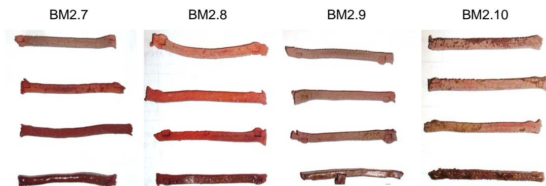
Figure 275: Samples BM2.7–BM2.10 after firing (top to bottom) to 800, 850, 900 and 950°C
