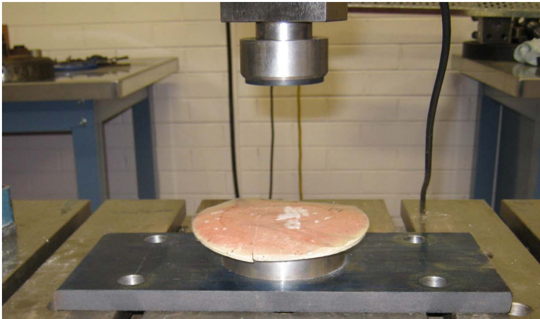
Figure 436: Ring stress test used for discs
