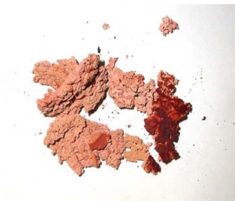
Figure 97: Corn seeper sludge calcined at 800°C
