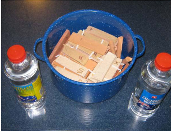
Figure 371: Dried and fired test bars separated with spacers prior to addition of distilled water
