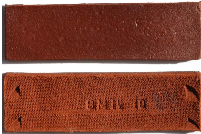
Figure 425: BM11.10 after firing to 1050°C: Exposed (top) and protected surfaces
