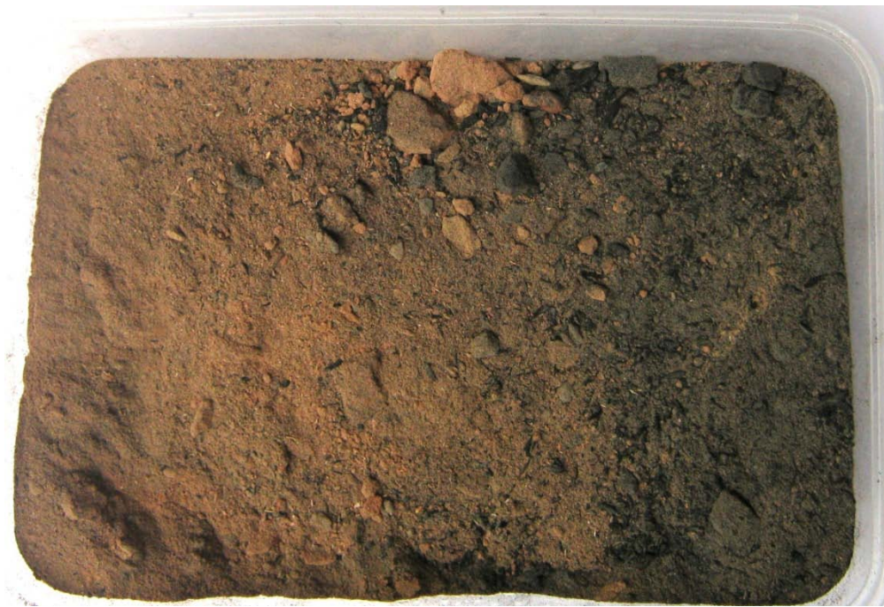
Figure 58: Bagasse ash (number 1 boiler belt) calcined at 800°C
