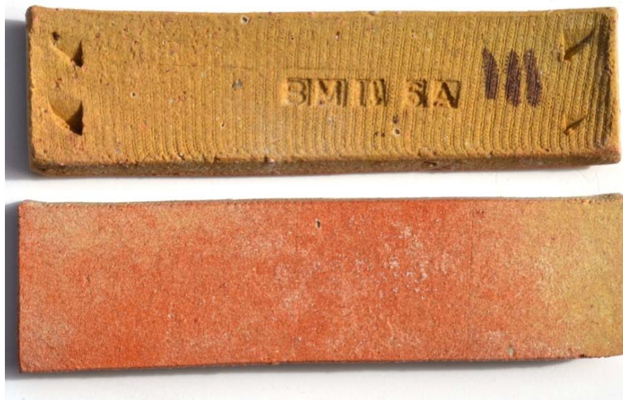
Figure 432: BM11.6A unglazed exposed side (top) and unglazed protected side after firing to 1050°C
