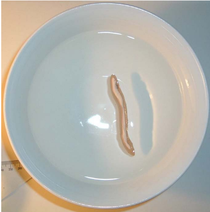
Figure 247: ACCL11 floating ceramic sample
