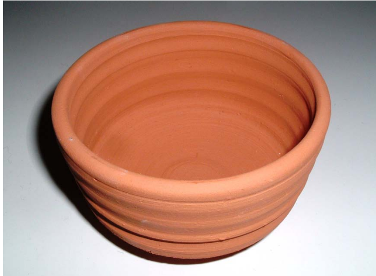
Figure 157: Bowl of 50% Bungendore, 50% Marulan tailings fired to 800°C
