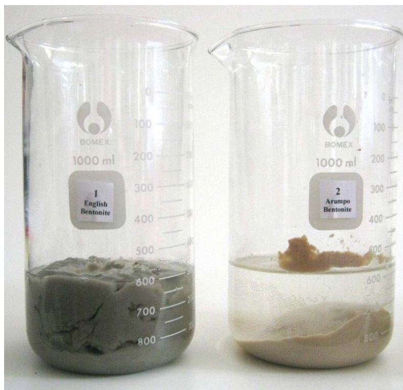
Figure 141: Water absorption of English (left) and Arumpo bentonites
