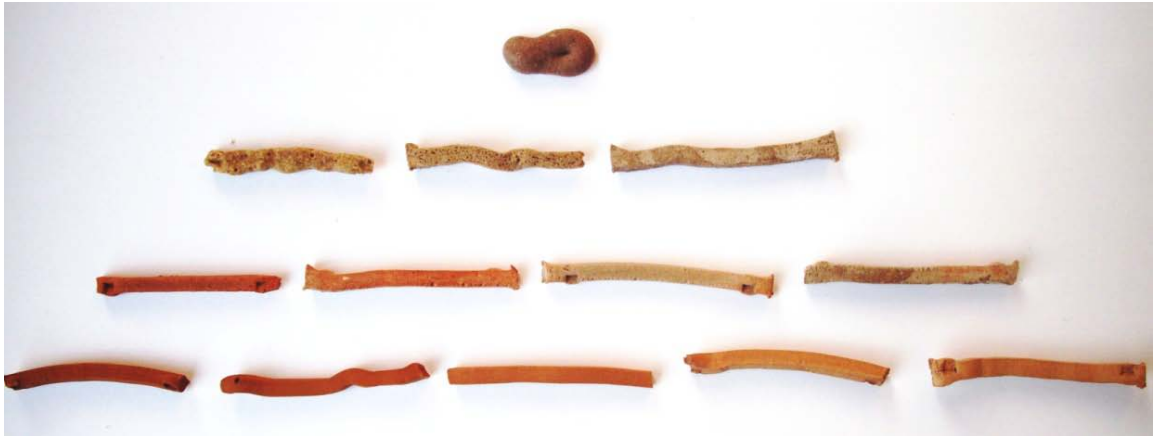
Figure 262: Triaxial BM2 fired to 800°C. Samples 3–15
