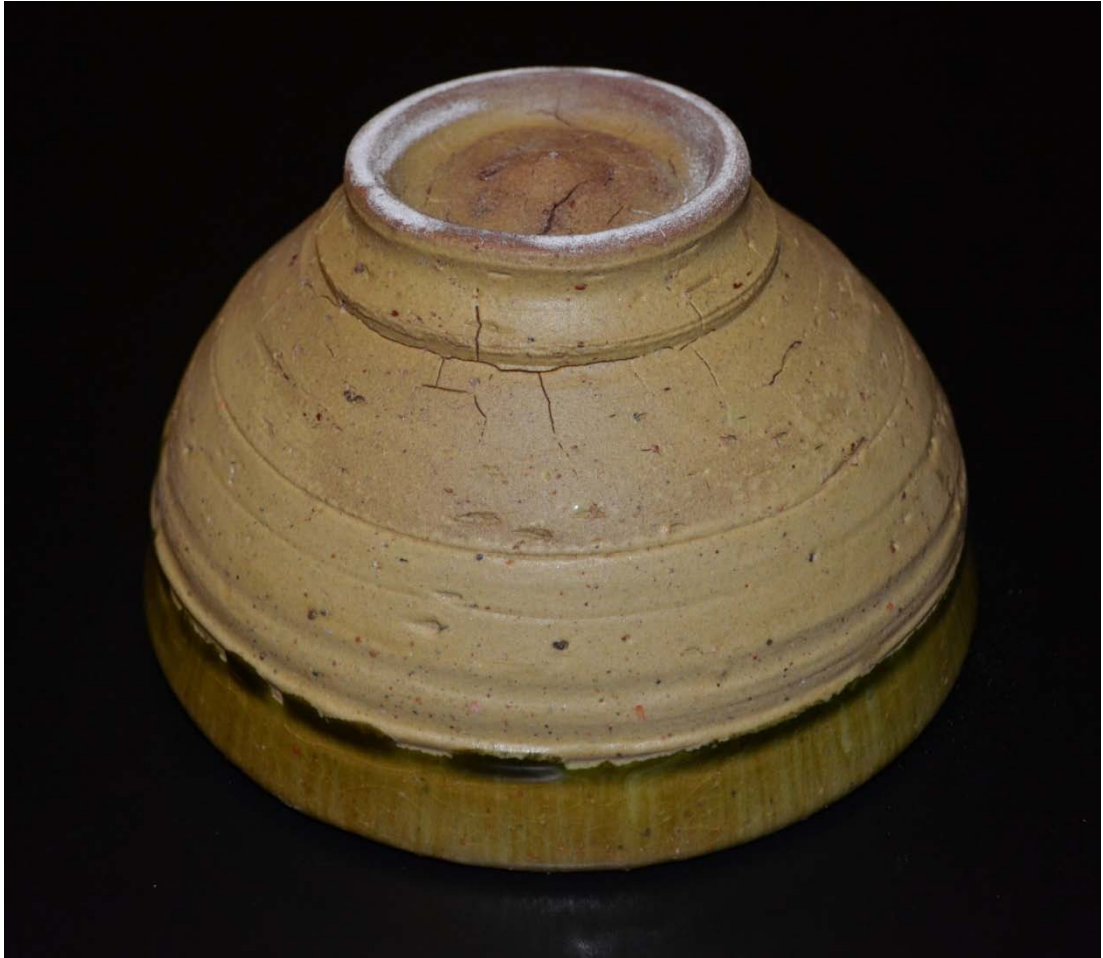
Figure 499: Bowl 4: BM11.6A, 950°C. Glaze 13.4 (rim). Self-glazed exterior, unglazed foot ring
