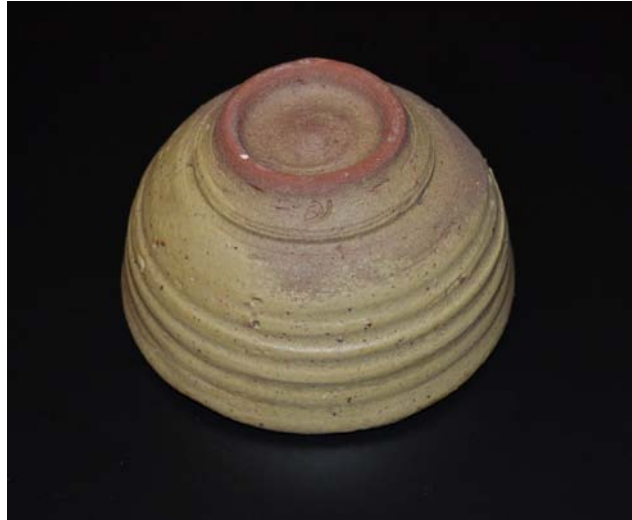
Figure 493: Bowl 2: BM11.6A, fired to 950°C, Self-glazed exterior, unglazed foot ring
