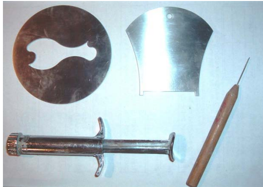
Figure 164 (clockwise from top left): Template, 50 mm profile, extruder, needle cutter
