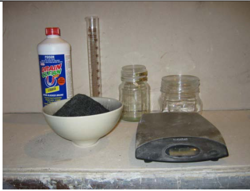
Figure 293: Equipment and materials for experimental production of sodium silicate
