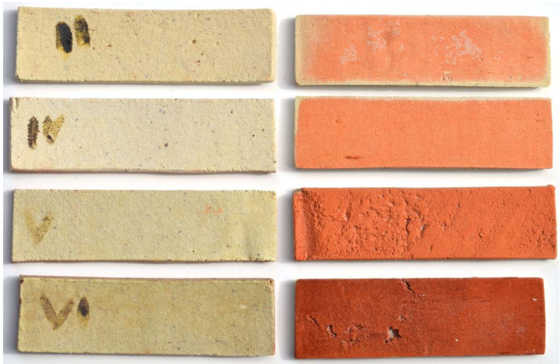
Figure 428: Effloresced exposed sides (left) and unaffected protected sides (right) of BM11.2 (top), BM11.4, BM11.5, and BM11.6 (bottom) after firing to 1000°C
