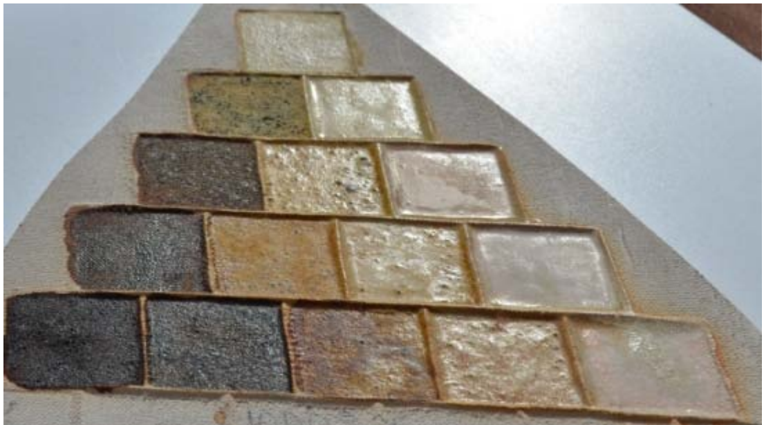
Figure 446: Reflectivity of glazes in triaxial low-fire 1 after firing to 1000°C
