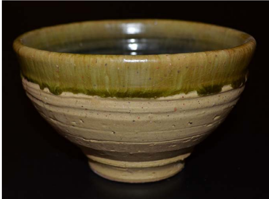
Figure 497: Bowl 4: BM11.6A fired to 950°C. Glazes 17.2 (interior) and 17.4 (rim)
