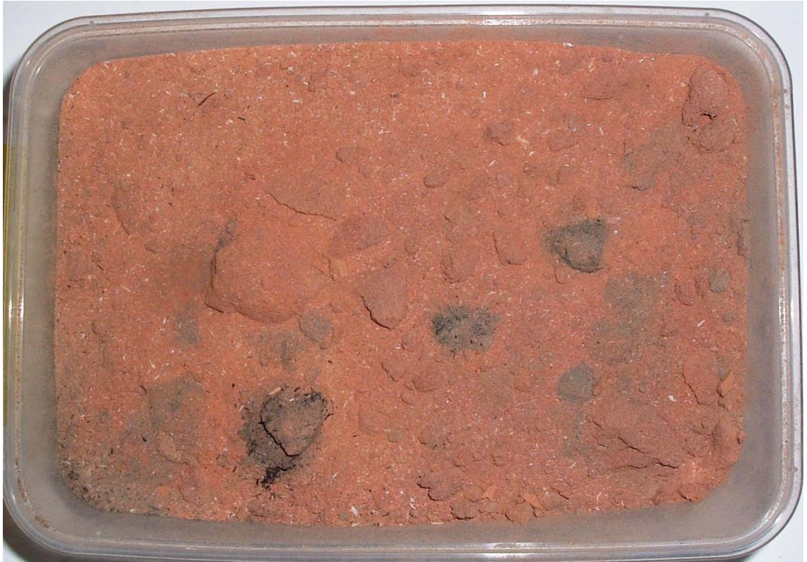
Figure 67: Bagasse ash (number 12 boiler belt) calcined at 800°C
