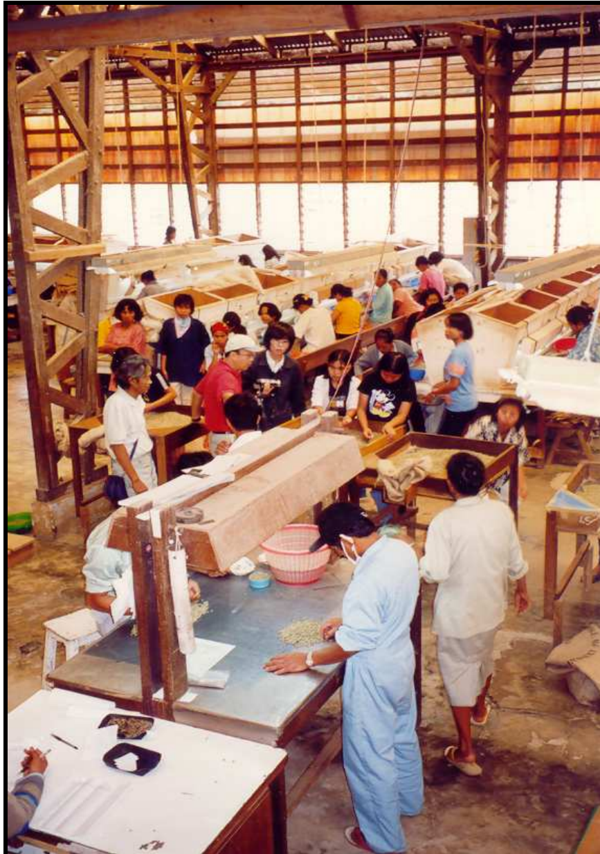
Plate 7-16 Hand sorting is still considered the most effective way of ensuring final quality
