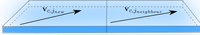
Figure 4.6 – Horizontally adjacent water current grid cells are expected to have similar water current velocities due to continuity [39].
