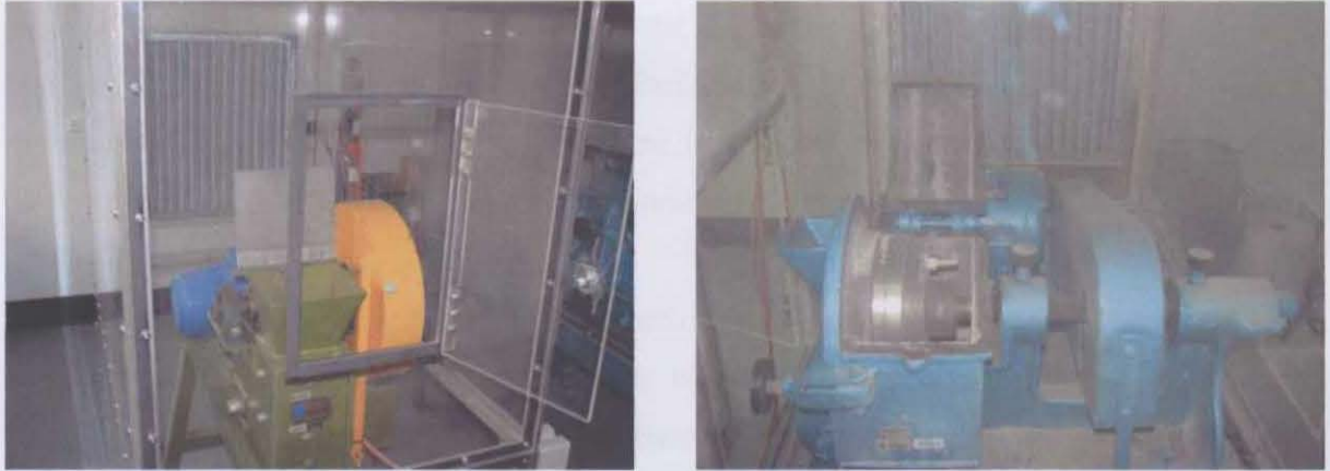
Fig. 4.4. Pre-treatment of soil parent materials. The photo on the left hand side shows a jaw crusher to crush rock samples to less than 2 cm and the photo on the right hand side shows a disc pulveriser to ground the 2 cm fraction to less than 500 \mu\text{m} (Source: ANSTO Sydney).
