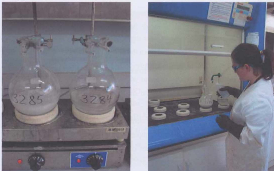
Fig. 4.5. Treatment with \text{H}_3\text{PO}_4 . The photo on the left hand side shows the point of white gel-formation resulting from external contaminants in the sample (Source: ANSTO Sydney).
