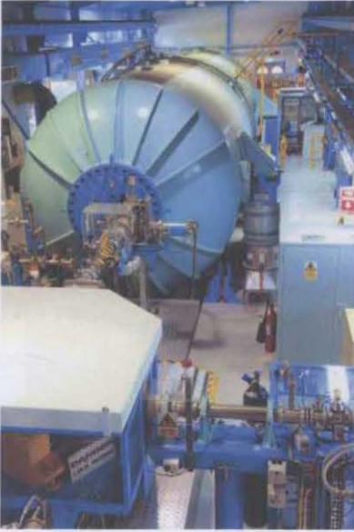
Fig. 4.3. The ANTARES AMS facility at Lucas Heights in Sydney, Australia. Photograph shows the 10MV tandem accelerator (Source: ANSTO Sydney).
