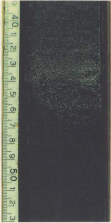
Figure 9.5: Photograph from Narrawallee core N5 showing erosional surface (20.1-20.3m) that marks the disconformity between Last Interglacial basin clays and Holocene tidal delta sands.
