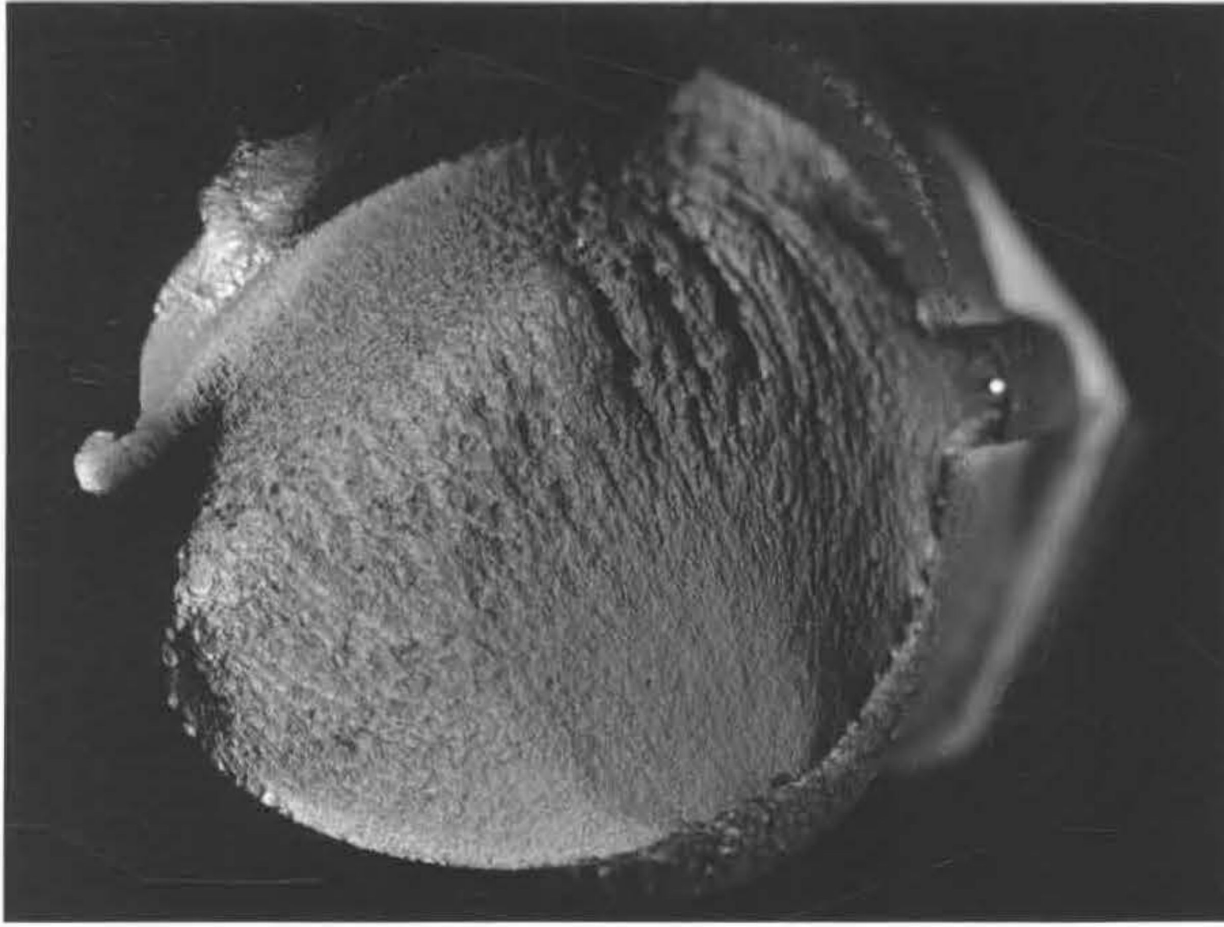
(a) single initiation at lug root (36 mm bar, \Delta\sigma = 250 MPa)
