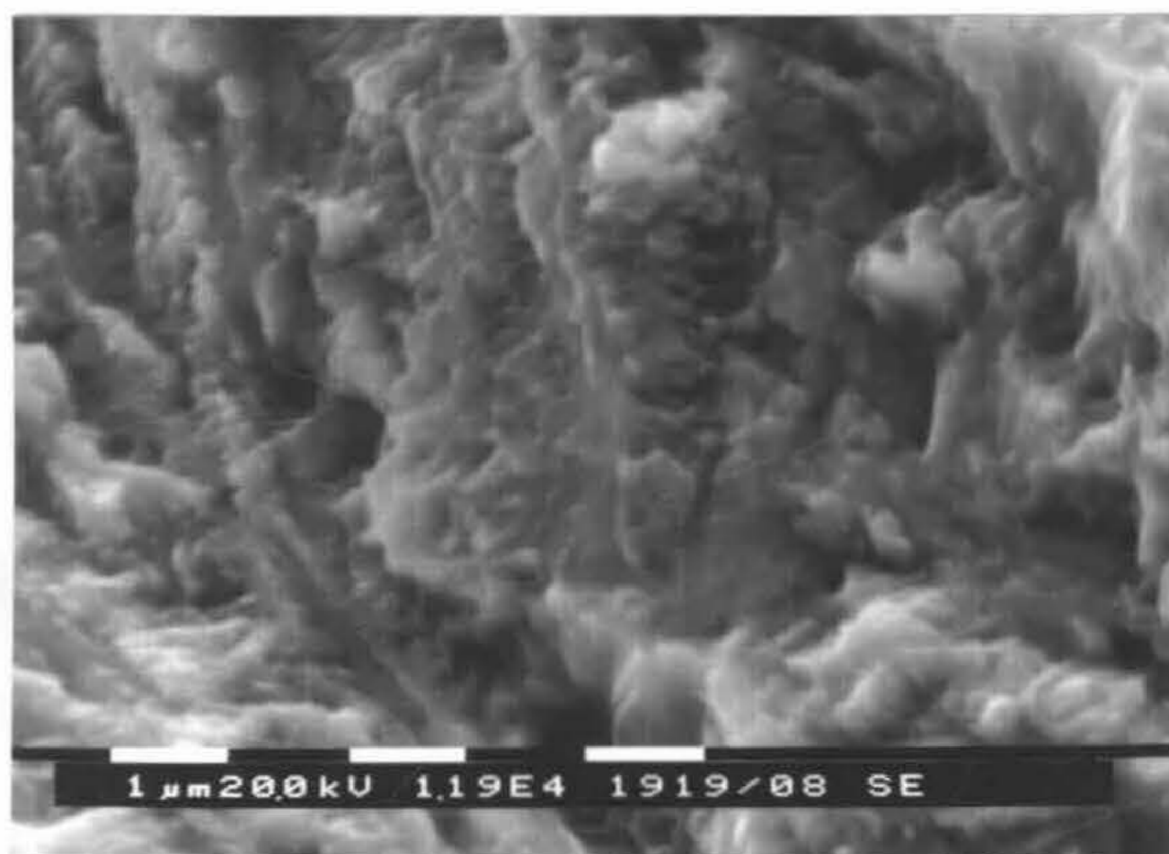
Figure 7-36. Fracture at 40 μm away from initiation point (16F340-1)
