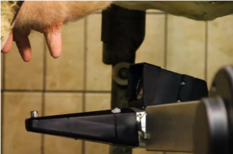
Figure 2.6: Post-milking disinfection of teats, the teat spray module (TSM; www.DeLaval.com )
