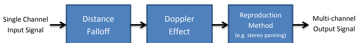
Figure 1. Signal Flow of Sound Source Motion Simulation.
