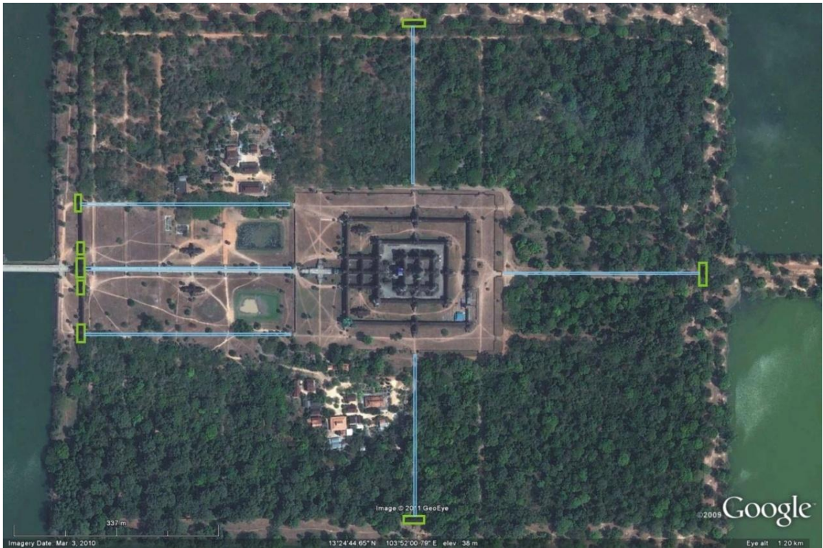
Figure 4.23 - The gopura (green) and their alignment (blue) with the central staircases; outer doorways of the West gopura and their alignment also shown. (Google Earth)
