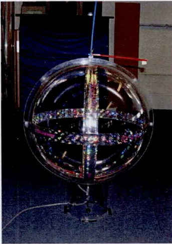
Figure 6.66. The long range Fastrak transmitter
