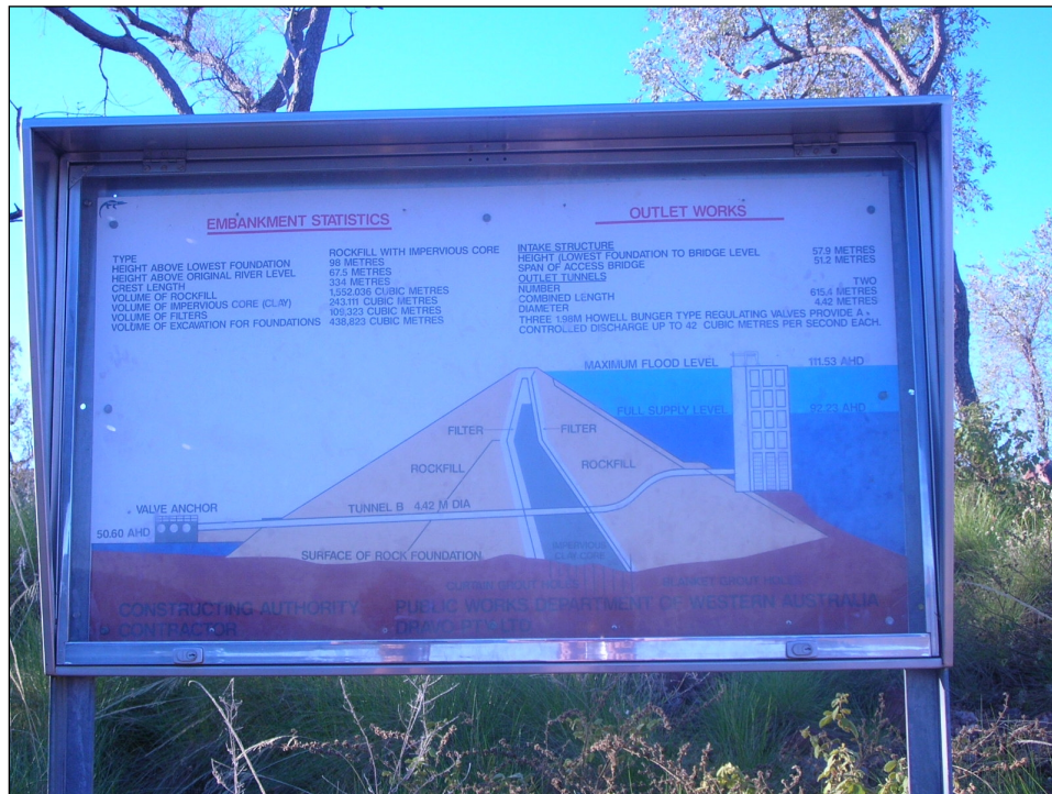
Figure Twelve: Sign showing how the dam works, overlooking Ord Main Dam.
