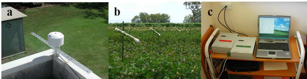
Figure 3.4. The installed BIOTIC equipment. a) receiver aerial and temperature and humidity sensor (inside Stevenson's screen) mounted on the edge of a building adjacent to the experimental field; b) BIOTIC sensors installed in field experiment; c) computerised base station data loggers.
