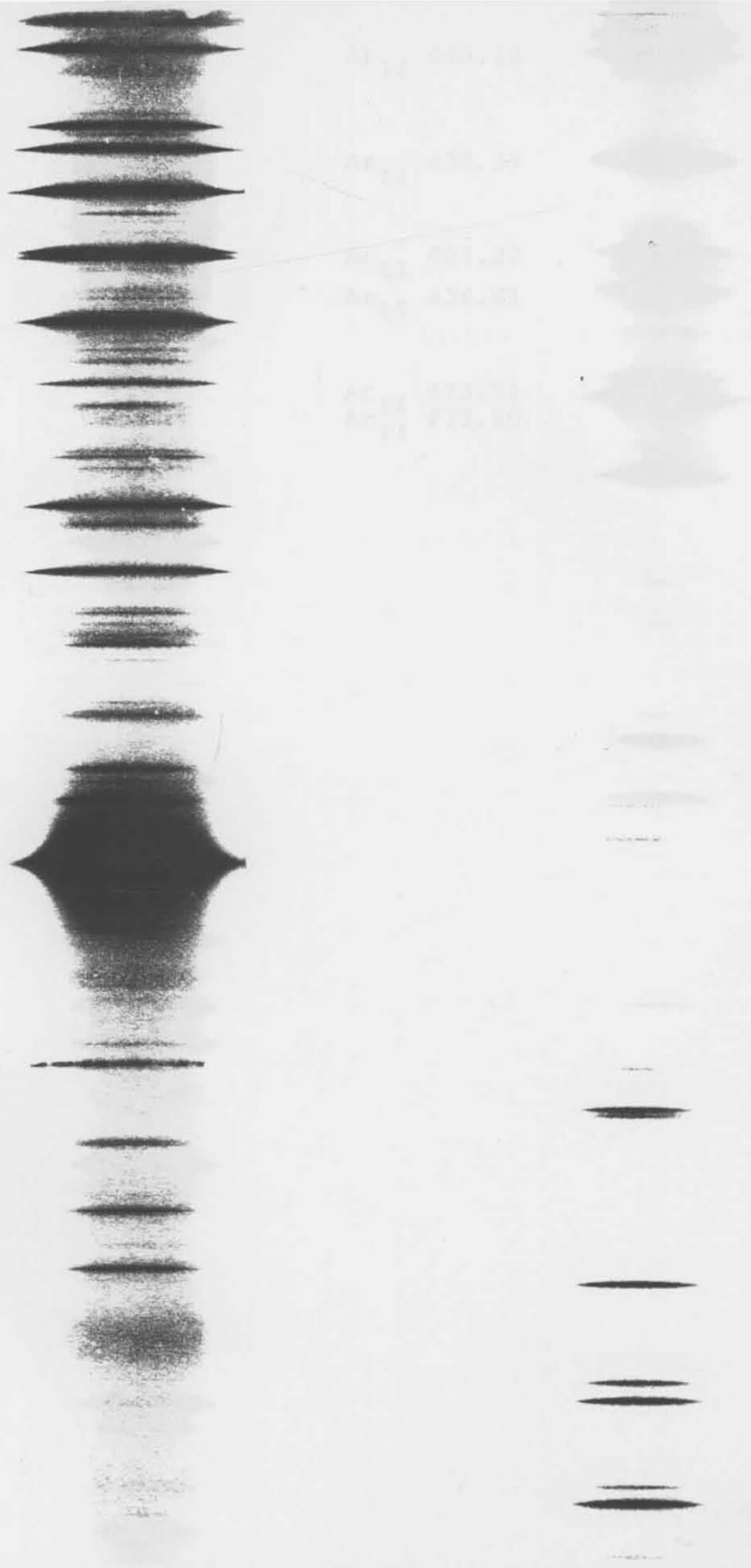
Figure 6.3: Argon arc spectrum (wavelength in nm). Arc current 424 amperes and pressure 1 atmosphere.
