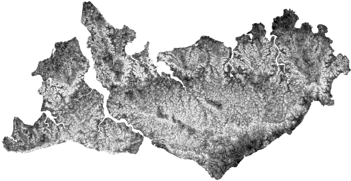
Figure 3-2 Static soil wetness index derived from 50 m DEM and classified into six quantiles
