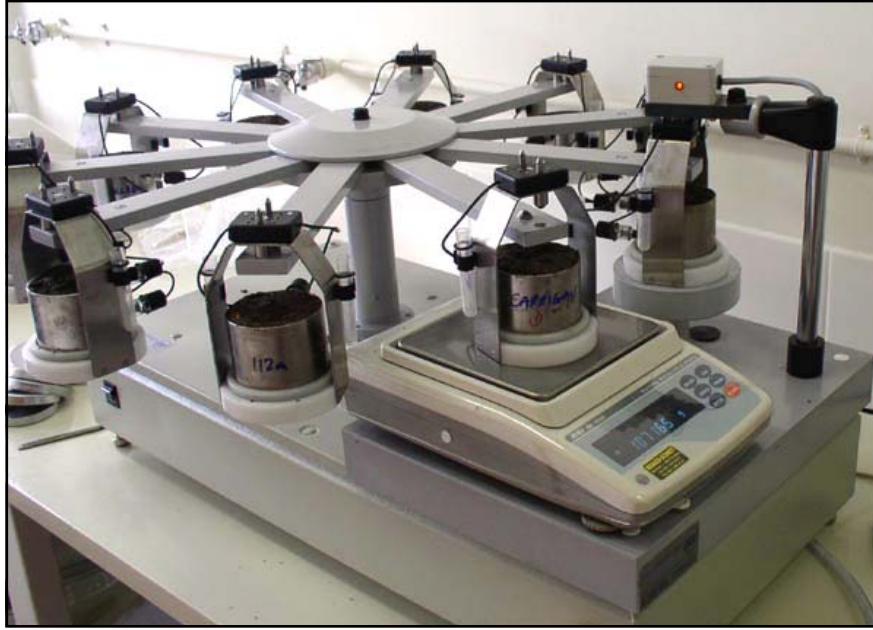
Figure 6.1 The ku/pF apparatus. Individual soil cores were hung in each of the ten baskets. This apparatus determines changes in matric potential and soil weight as moisture evaporates from the surface of individual soil cores.
