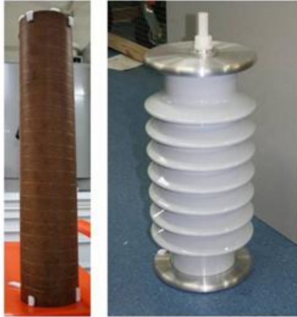
8-7 Left: Press board tubing and coiled double flat fibre, Right: Porcelain insulator and end electrode plates.
