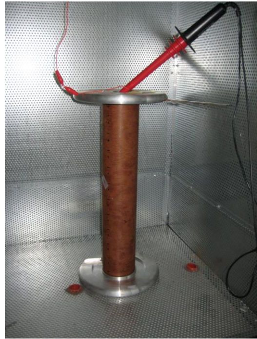
8-8 Left: Magnetic voltage transformer used to both generate and monitor the test voltage, Right: A coiled sensor being tested without the porcelain insulator.
