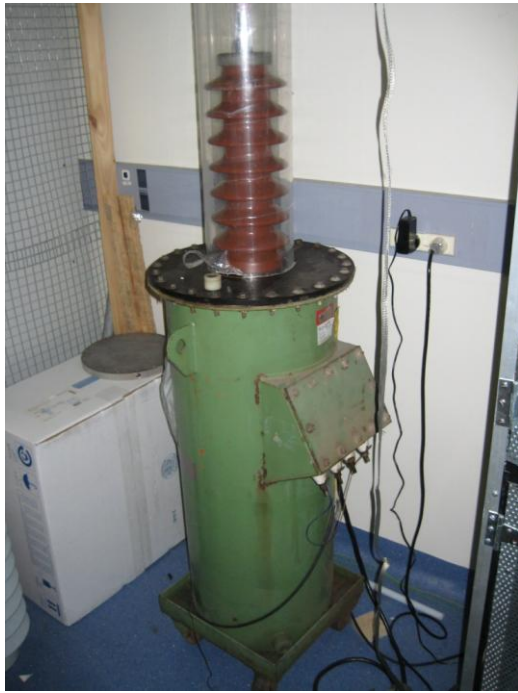
8-8 Left: Magnetic voltage transformer used to both generate and monitor the test voltage, Right: A coiled sensor being tested without the porcelain insulator.
