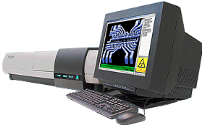
Figure 3 Skyscan 1172 Desk Top microCT X-ray scanner
