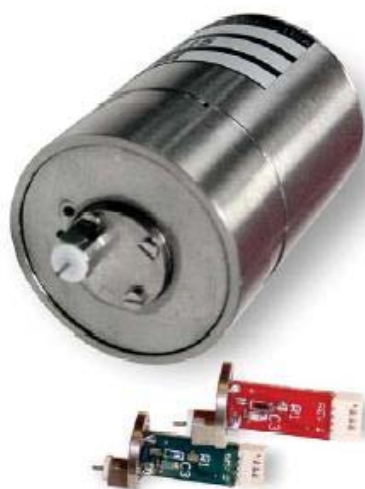
Figure 2-4: The Molecular Imaging's (Agilent's) STM scanner with two additional interchangeable pre-amplifier modules. One pre-amplifier module contains the logarithmic amplifier used to observe currents ranging from metallic conduction to molecular conduction observed during break-junction experiments (i.e. ranging from 10^3 to 10^{-5} G 0 , depending on the applied bias.) 75
