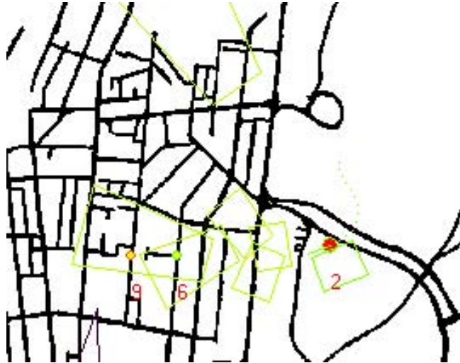
Figure 5.2: The Finite Horizon Footprint chasing control scheme for a 5 second look ahead planning horizon. Predicted footprints are shown in light green with the dark green indicating the current footprint. The UAV bank angle control associated with the footprint providing the best \sum_{x \in s} V_{xnet} is chosen for the current planning cycle.
