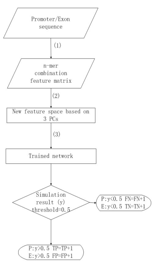
Figure 3.6 The flow chart of the testing process
