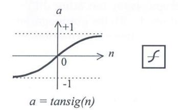
Figure 3.4 The figure of tan-sigmoid transfer function
