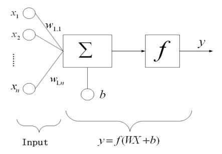
Figure 3.2 The structure of a general neuron.
