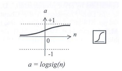
Figure 3.3 The figure of log-sigmoid transfer function
