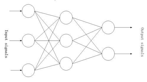
Figure 3.1 Schematic illustration of an ANN
