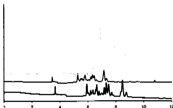
Figure 11. Charge-based separation of high- and low-molecular-weight glutenin subunits in the Beckman MDQ. Top - combined, middle - LMW subunits, bottom - HMW subunits.
