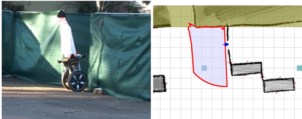
(a) The robot must lean forward to accelerate (b) Leaning causes the laser scan to intersect with the ground
