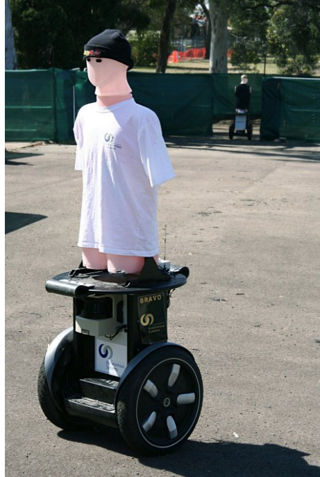
Figure 1.3: A robot and its environment. The robot is dynamically stabilised. A forward-looking scanning laser range-finder is mounted centrally, just above the wheels. A second robot is in the background.
