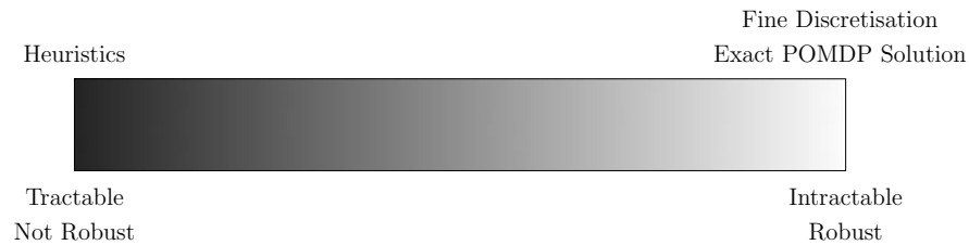
Figure 1.1: POMDP solution methods span a continuum. On one extreme, the combination of a fine discretisation with exact value iteration will produce excellent plans but will be incapable of scaling to realistic problems. On the other extreme, heuristics require little computation but fail to take a principled approach to uncertainty. The most useful planner lies somewhere in the middle. The figure is adapted from [94].
