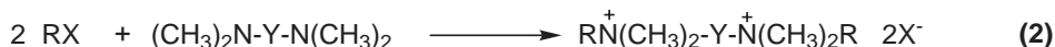
Figure 1.5: Common synthetic routes to cationic gemini surfactants; the R-group becomes the surfactant tails, the Y-group the spacer and X – a halide – the counterion.
