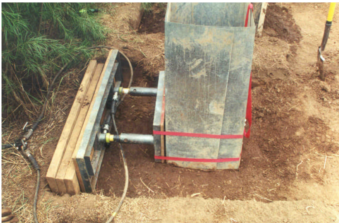
Figure 5.2: In-situ shear test apparatus in a trench between a soil block ready for testing and the greater soil mass. The pushing plate is strapped adjacent to the metal form guide that contains the soil block and normal load.
