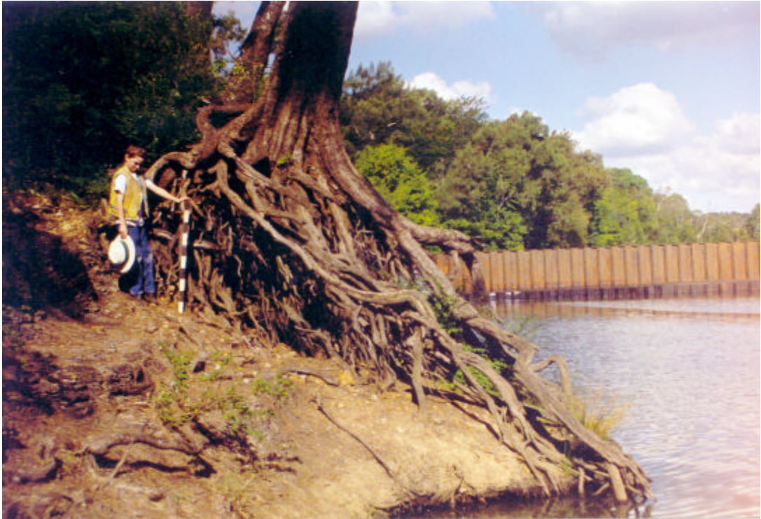
Figure 3.15: A mature Casuarina tree growing within the study area. Despite the presence of bedrock and washing away of the bank sediments, many of the comparatively large roots re-enter the bank face at a depth of around 1.7 m below the original ground surface.
