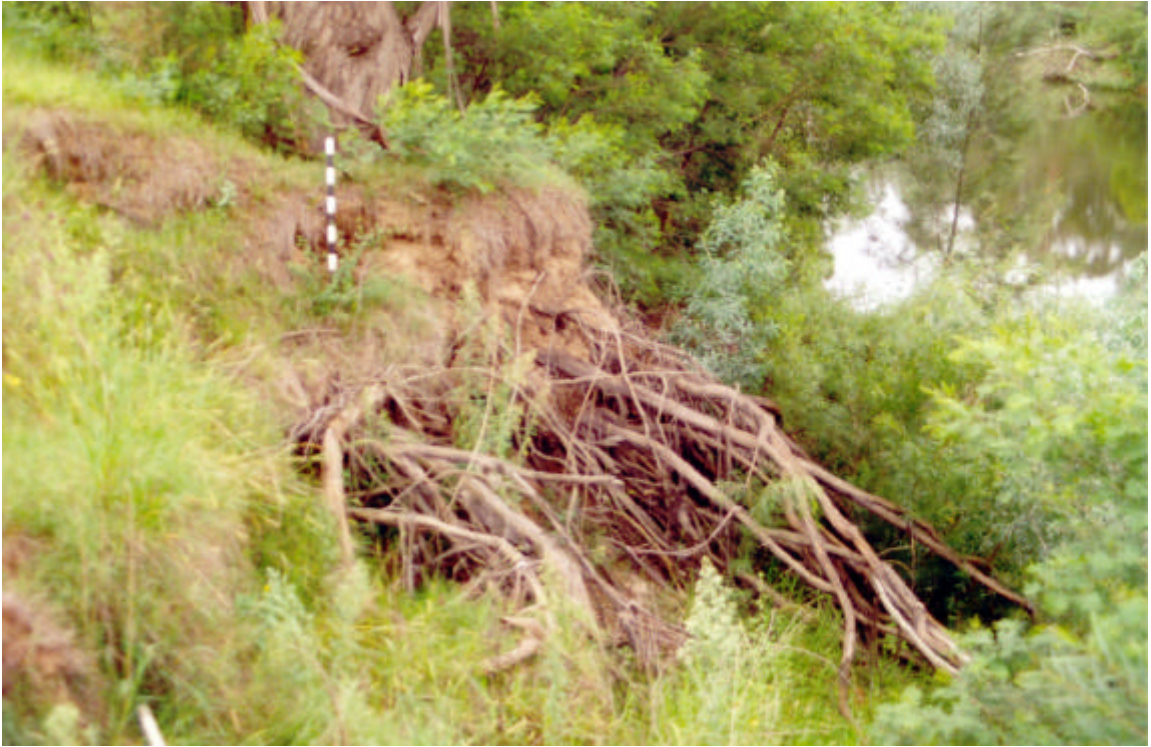
Figure 3.13: A mature Eucalyptus tree growing within the study area. Note the exposed root system in the failure scarp where it is possible to observe large roots re-entering the bank material directly below the tree stem at a depth of approximately 4 m below the ground surface.
