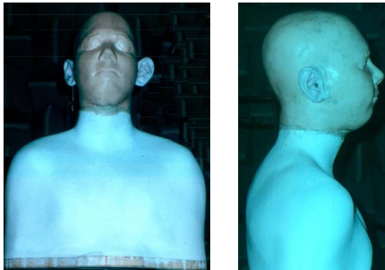
Figure 1: A life-like acoustical mannequin was made.
