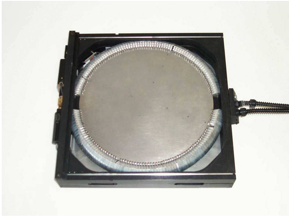
Figure 3.2 The 6dF field plate. The buttons are all in the park position. The retractors can be seen as a metal ring around the outside of the plate. One of the cables leading out to the right take 150 science fibres to the spectrograph and the other cable contains 4 guide fibre bundles.
