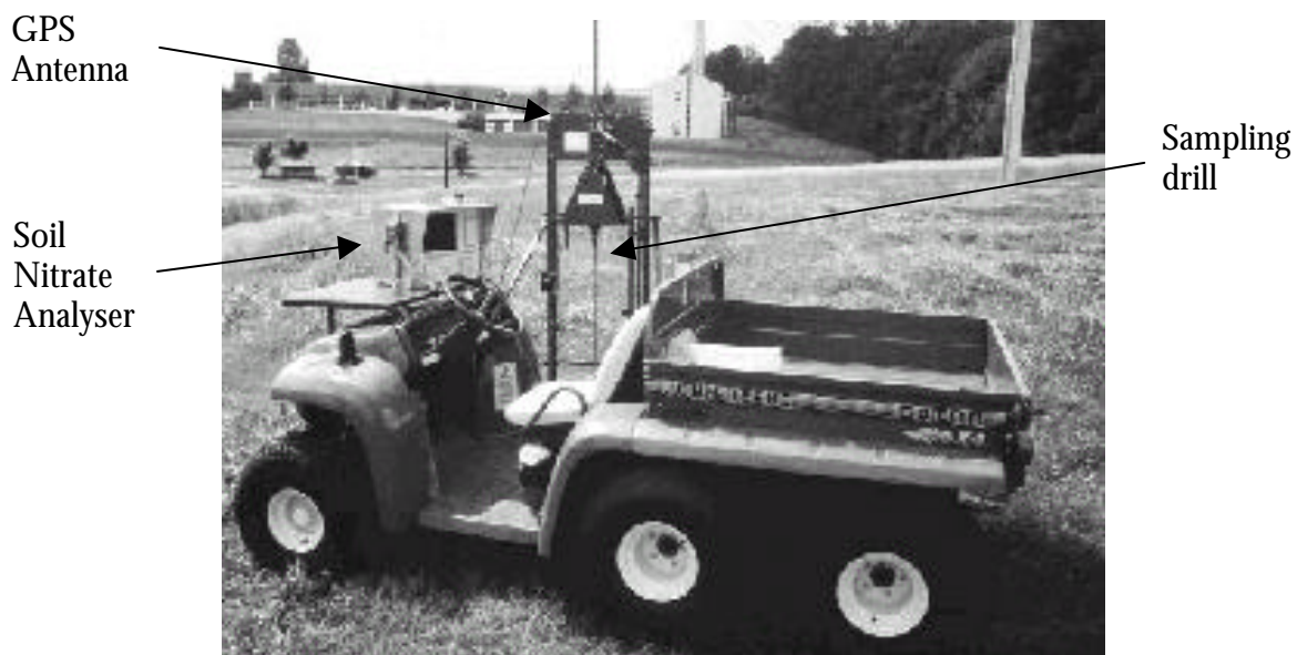
Figure 2.5 Field-based automated soil sampler and nitrate analysis system of Wild et al. (1997)
