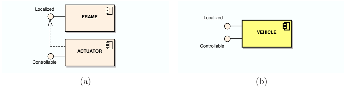
Figure 3.38: A custom VEHICLE component: (a) canonical implementation using a FRAME and a ACTUATOR and (b) custom implementation. The localization service provided by Localized interface to ACTUATOR is internalized inside the custom component but both interfaces must still be provided for the benefit of other components in the system. Notice that the interfaces remain unchanged.
