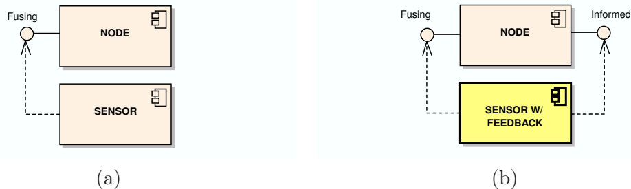
Figure 3.41: A custom SENSOR component with state feedback. The environment information from the NODE component is made available to the custom SENSOR through the Informed interface. All interfaces remain unchanged.
