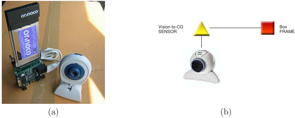
Figure 6.14: A stationary webcam with a processing unit: (a) the physical view and (b) the component diagram.
