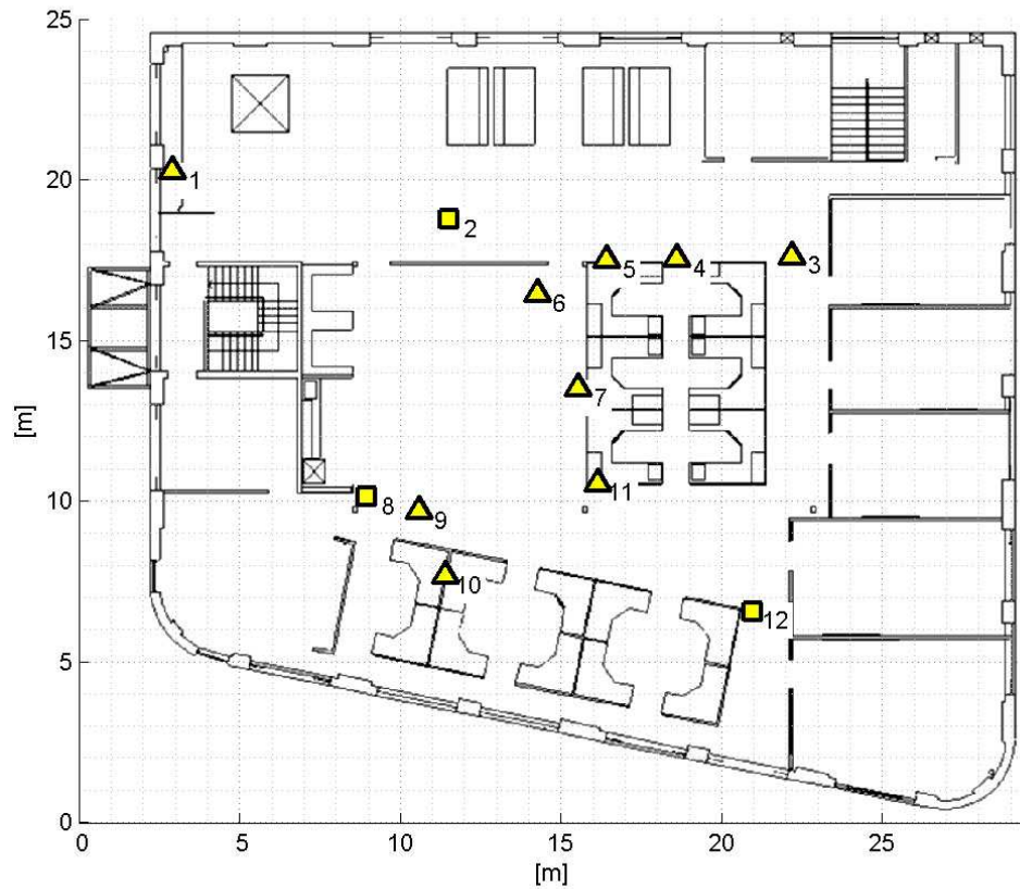
Figure 4.26: Deployment of sensors in the motion mapping experiment. The experiment employed a total of 12 sensors of two types: lasers ( \square ) and video cameras ( \triangle ).
