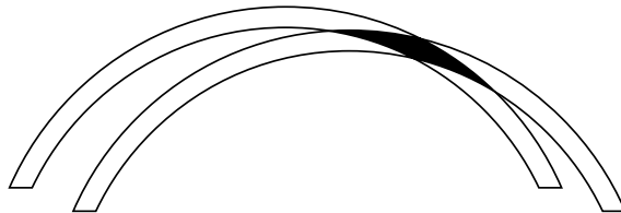
Figure 3.4: The rhombic area of overlap between two spherical pupil caps.
