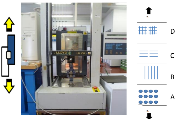
Fig.2- The shear load test machine (sx) of the four types of laser welded polymeric joints (dx).
