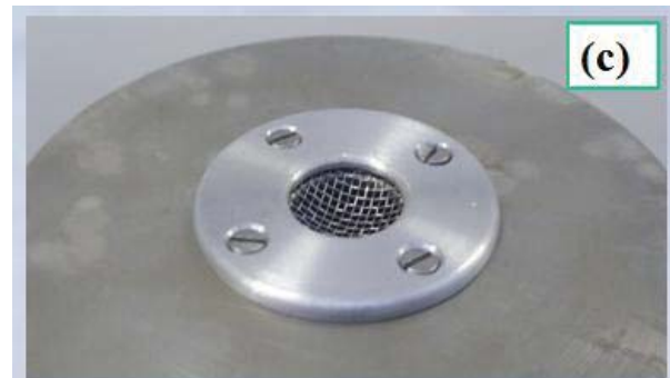
Figure 2: Photos of the extraction hole without a grid (a), with a plane grid (b) and with a curved grid (c).
