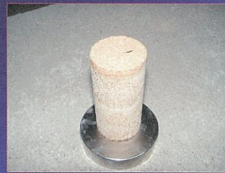
The decomposed granite soil with the gypsum mixing \phi=50\text{mm} H=100\text{mm}
