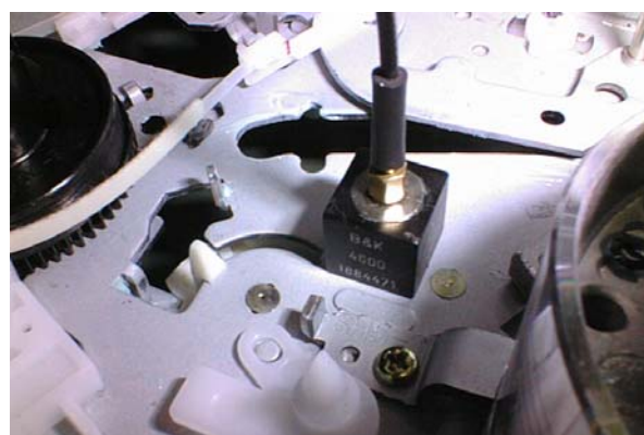
(c) The accelerometer set near the gear.
