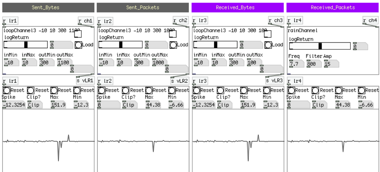
Figure 6: This screen grab shows a series of spikes in the sent bytes and received bytes variables. The audio file multiSpike_1s.wav demonstrates how this sounds at a playback speed of 1 s per record using signed log return values. There is an audible difference between the positive and negative traffic changes. However, notice how the peaks are not salient when playing back signed values at the faster rate of 20 ms as in multiSpike_20ms.wav — the peaks occur at around the 1.5 s mark in the audio file.
