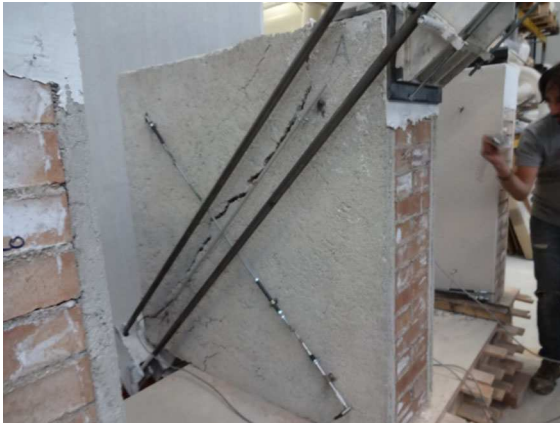
Fig. 7 Reinforced panel after failure (panel reinforced with mortar Type D)
