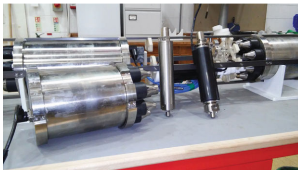
Figure 13. Sample containers used in the probe for recovering water samples. (Online version in colour.)
