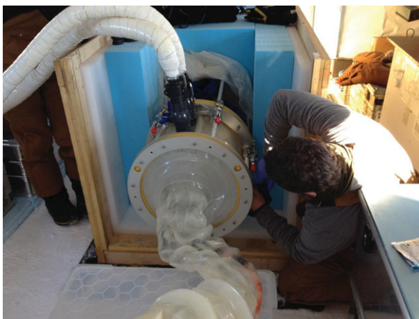
Figure 4. Probe handling in field and laboratory conditions. Attachment of the probe to the tether inside a portable glove box in the field. (Online version in colour.)
