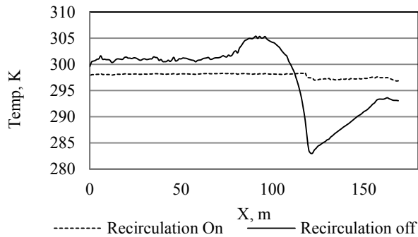
Fig. 4. Temperature variation with and without re-circulation at Y=0.6H_1 , Z=0.3W .
