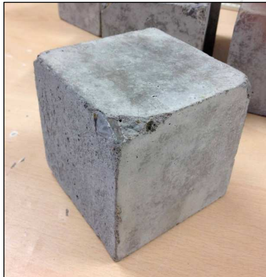
Figure 7 – Batch ‘A’ surface at final scaling inspection (70 cycles)
