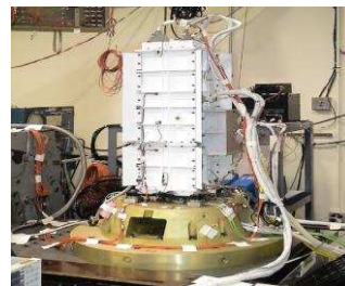
Figure 2.9 An advanced Stirling Radioisotope Generator (ASRG) 130-140 Watts unit which utilises plutonium-238 as heat source developed by NASA [6]
