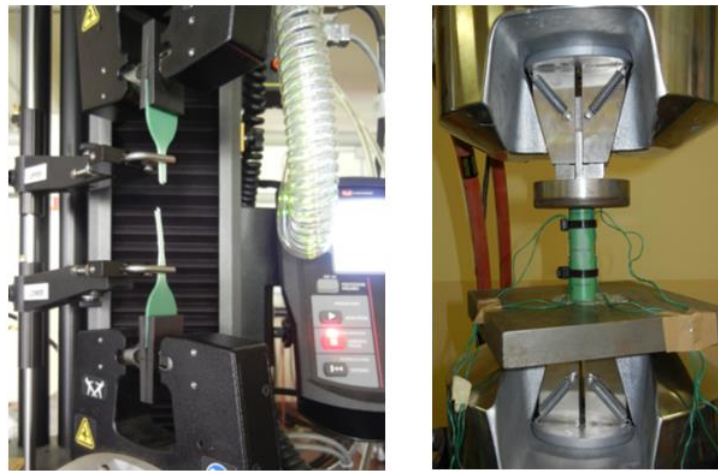
Figure 7 Tension (left) and compression (centre) tests on polyamide specimens
