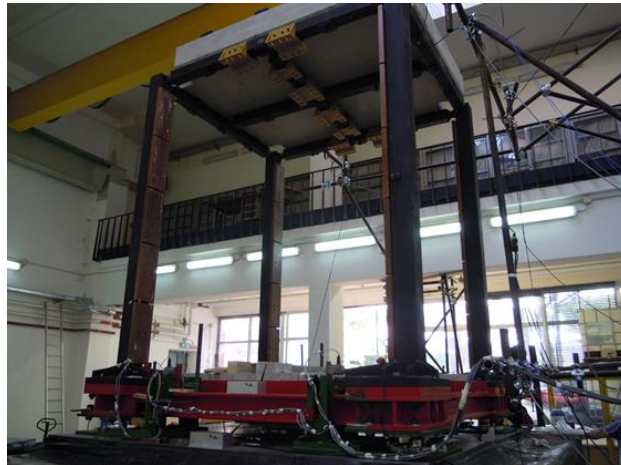
Figure 10 Shake table test set-up
