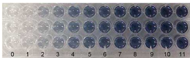
Fig. 1 Reaction of OPA reagent with ammonia (concentration of NH 4 Cl standard solution in mM indicated as number) after dilution with DMSO.
