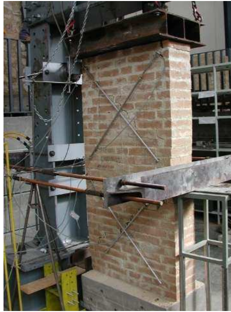
Fig. 3 Typical layout of a shear-compression test.
