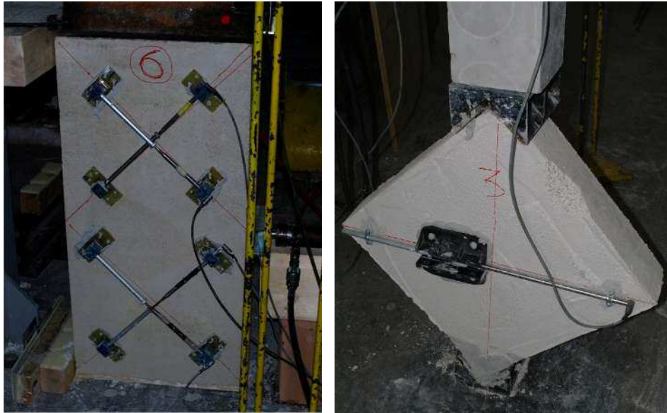
Figs. 5-6 Diagonal compression and shear-compression tests carried out on mortar small-scale panels.
