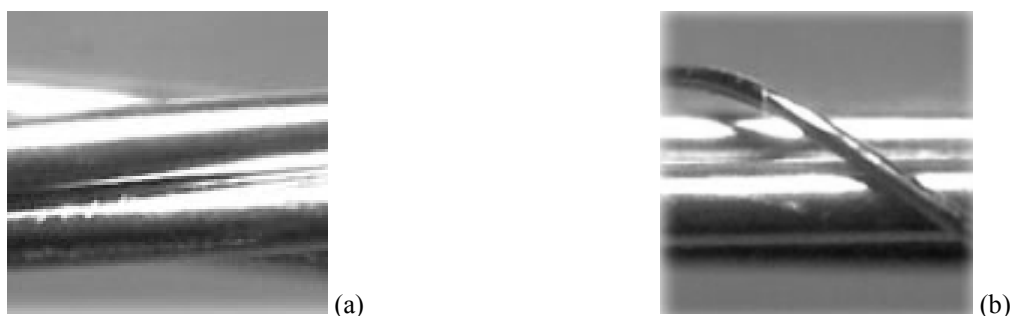
Figure 2. (a) 3X2 cord (Type 2); (b) 3SX cord (Type 1).
