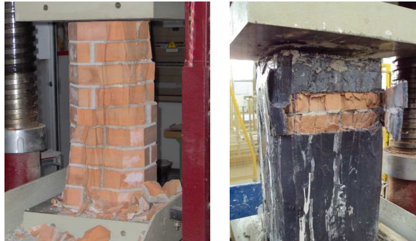
Figure 7. Failure modes of square cross-section column: (a) unreinforced specimens; (b) reinforced specimens.
