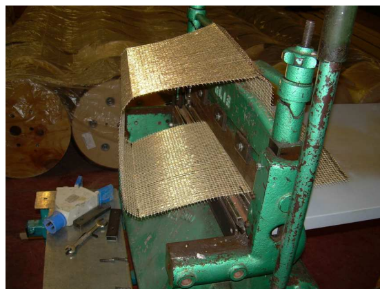
Figure 4. Cord cold bending (used only for square cross-section columns).
