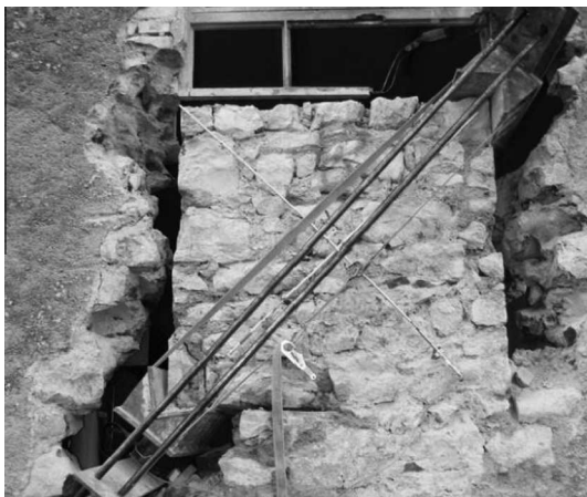
Fig. 9. Un-reinforced panel tested at Colle Umberto.
