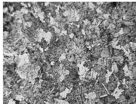
(a) variant 1 rolling according to LWM
