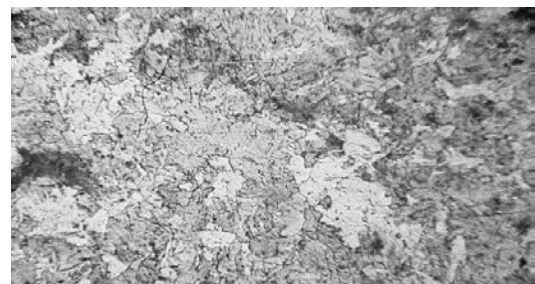
(c) variant 3 rolling according to LWM
