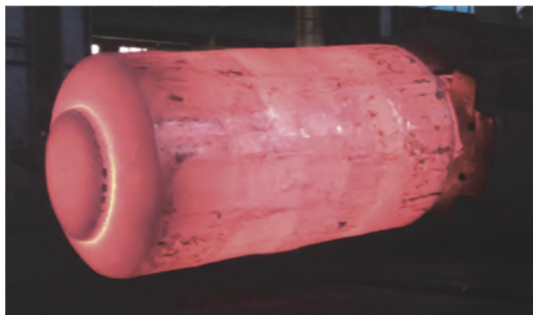
Figure 9 End-face produced with improved process
