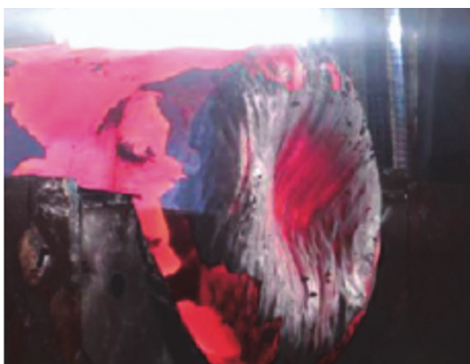
Figure 1 Dent on the end-face of the forging
