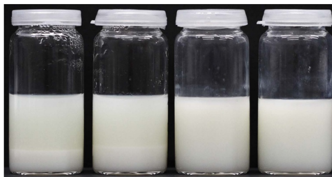
Figure 5. Macroscopic behaviour of the four different hydrocolloids dissolved in milk (0.1 wt% hydrocolloid). From left to right: xanthan gum, guar gum, iota-carrageenan and gellan gum. Xanthan gum and guar gum show a phase separation whereas iota-carrageenan and gellan gum do not.
